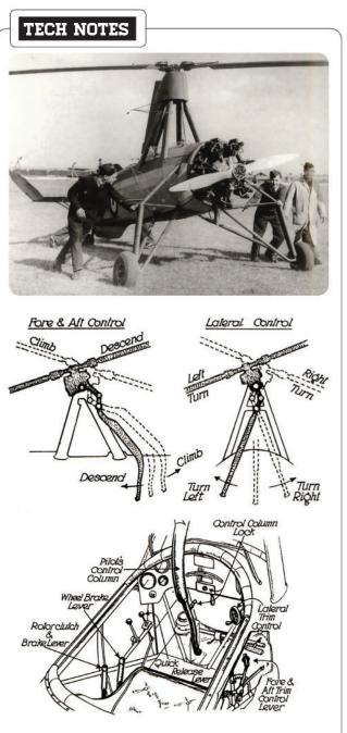
**KEY TO CONTROL** The C.30A/Rota I (shown at top being rolled out for a radar calibration mission) featured a long control arm attached to a tilting rotor mount (illustrated above) that gave pilots direct control over the Autogiro's movements and greatly improved low-speed handling.
