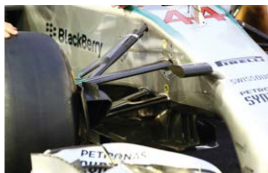
The suspension of the car has been defined by aerodynamic factors. Note the unique lower wishbone design
