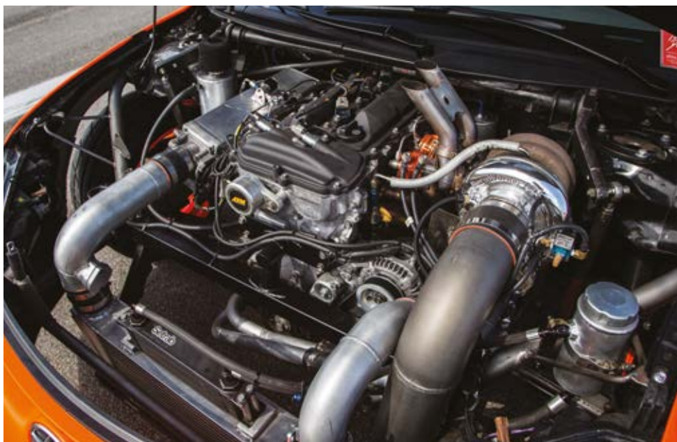
The Scion's longitudinally mounted turbcharged engine runs on nitrous oxide
