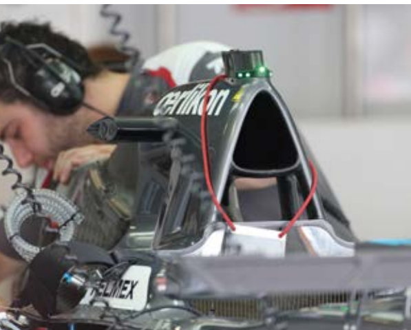
Roll hoop with lights and camera housing. 'The need for cooling on these cars is remarkable compared with the past'
