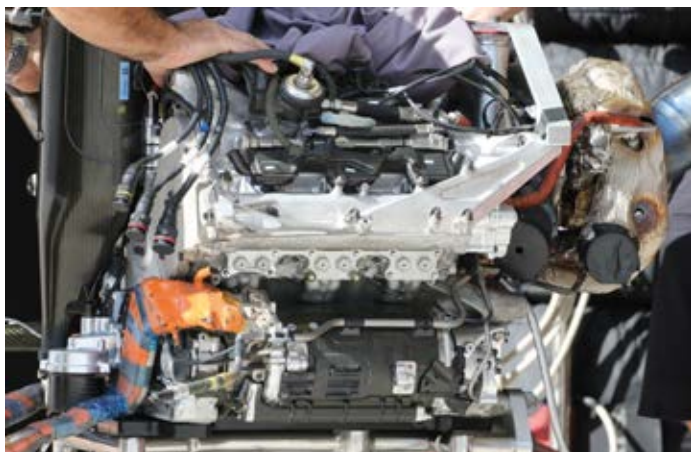
The Renault RS34 V6 engine showing clearly its turbocharger
