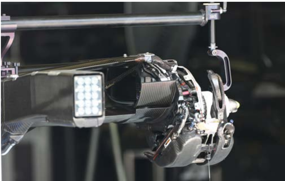
The car's rear brake setup with aerodynamic elements added
