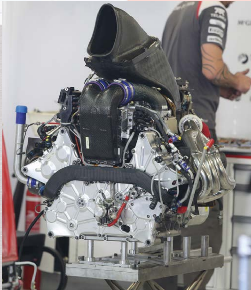
The Ferrari 059/3 1.6 litre six cylinder single turbo power unit
