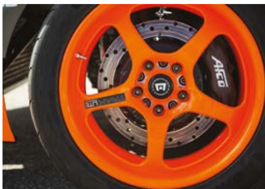
The wheel. Brakes are not heavily taxed so can be light-duty
