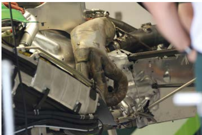
Renault RS34 exhaust manifolds believed to use Sulzer-type GDR
