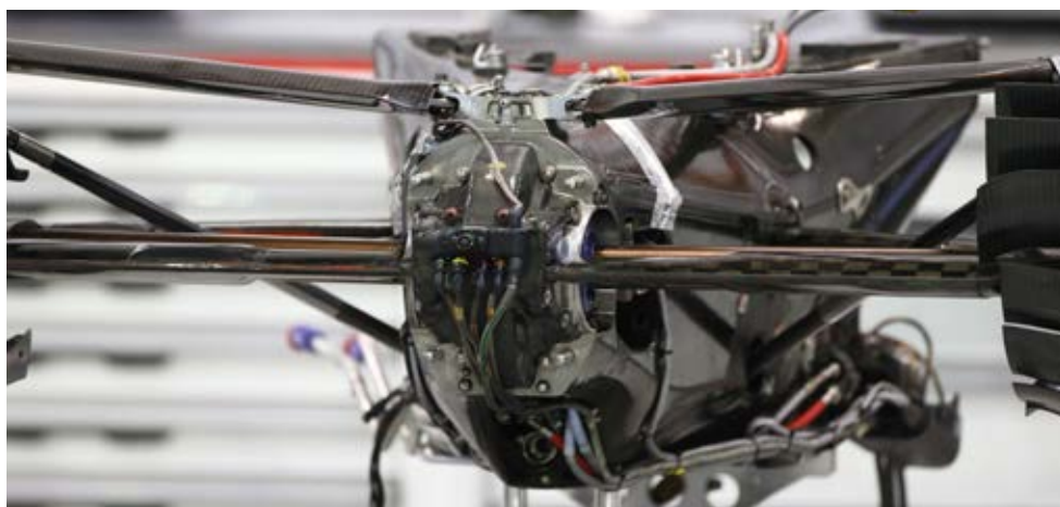
Sauber's transmission, as supplied by Ferrari, with rear crash structure removed
