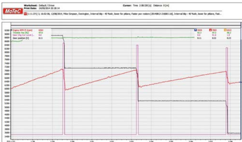
Above: data trace illustrating the upshift sequence of a Ginetta G55 GT4. The selector barrel trace (black) moves smoothly between each gear and the rpm trace (red) is uninterrupted with minimal 'ringing' after each shift has been completed, demonstrating clean and smooth shifting.
