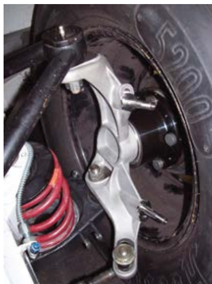
A NASCAR stock car spindle manufactured by CRP Group
