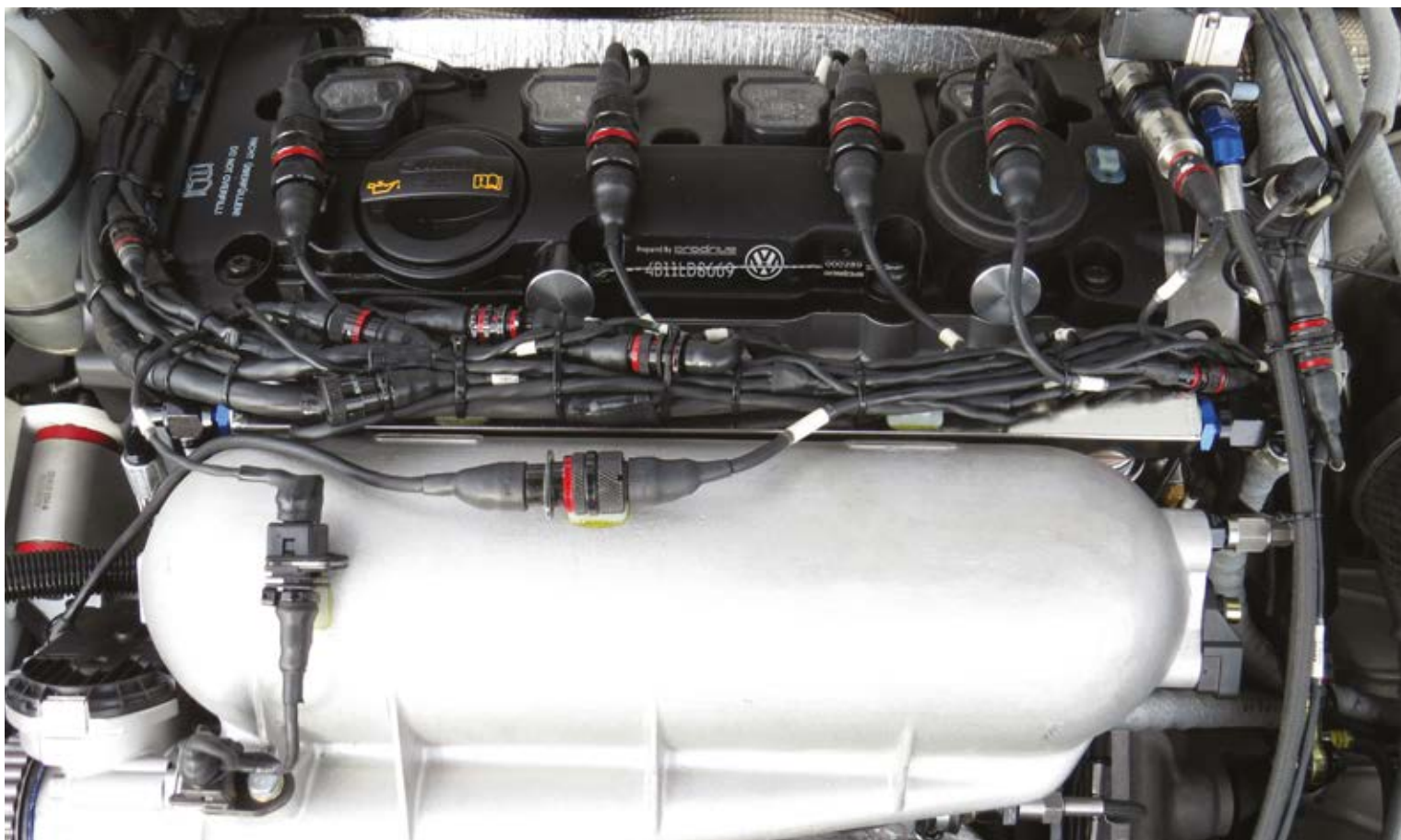
A production-based 2.0-litre four-cylinder VW engine powers the car. Prodrive have used all their experience to create this rally Golf. Post-MINI, it's clearly evolved – and it's got a bigger engine
