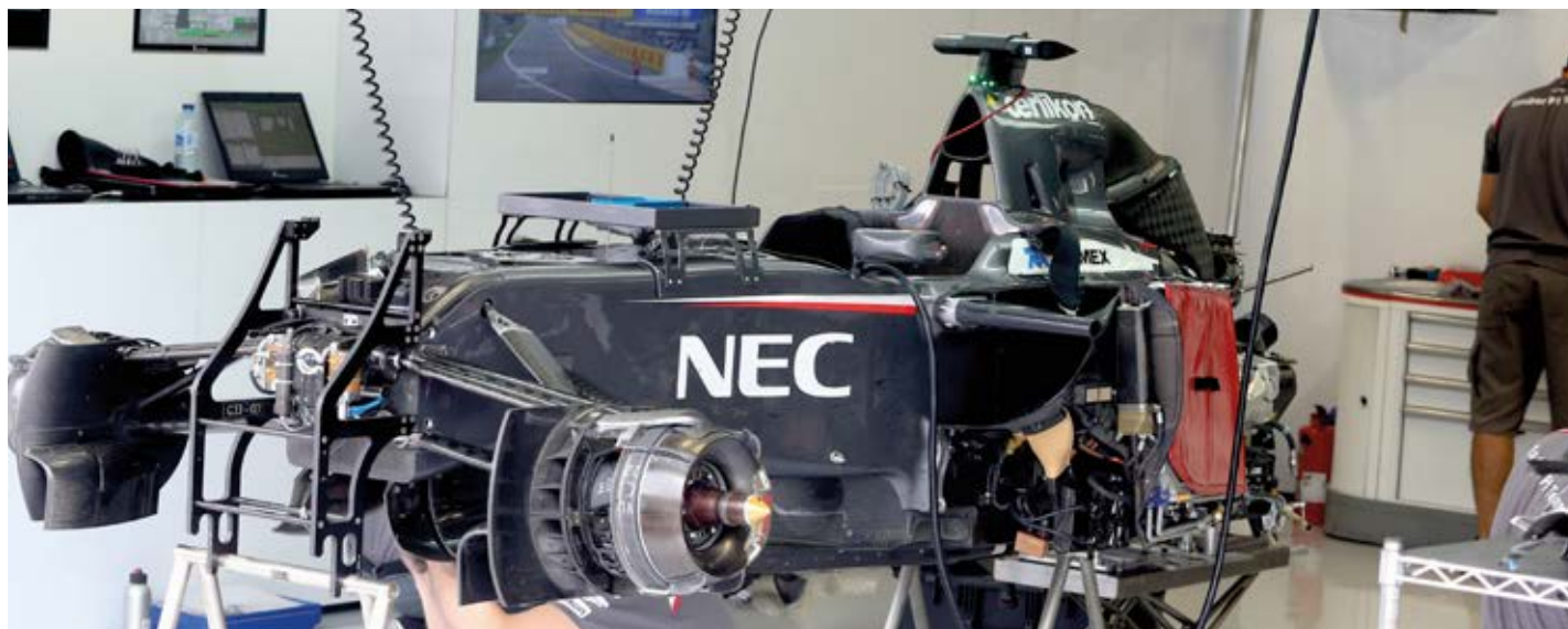
The Sauber chassis, fully built up but with rear end and nose removed. 'The car overall as a package is our worst in a while'
