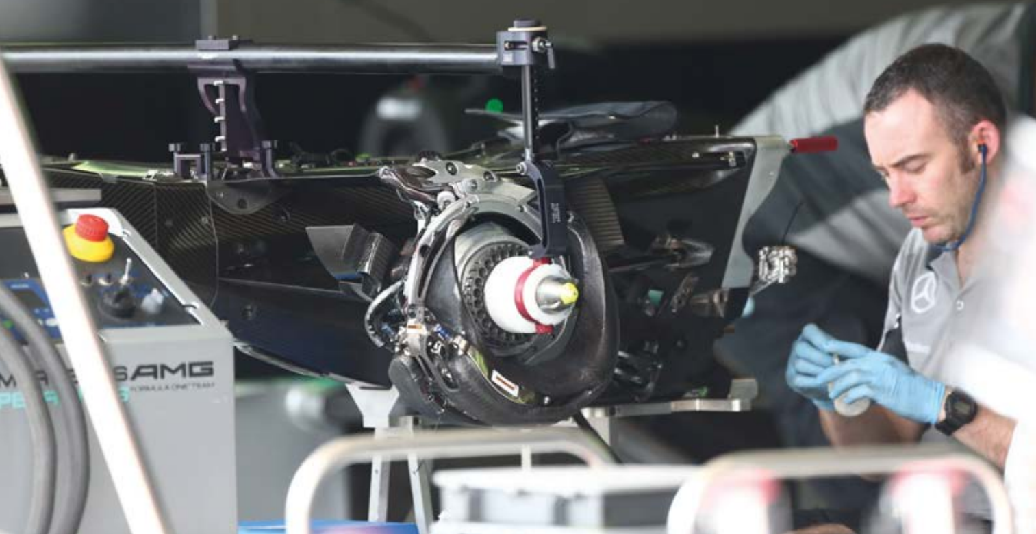
The W05 Hybrid gearbox features a carbon fibre outer case and titanium inner. Note also rear brakes setup
