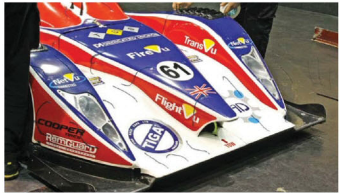
Picture 5: Tiga A's concave nose; compare to the gentle convex shape inboard of the wheel pods in Picture 3
