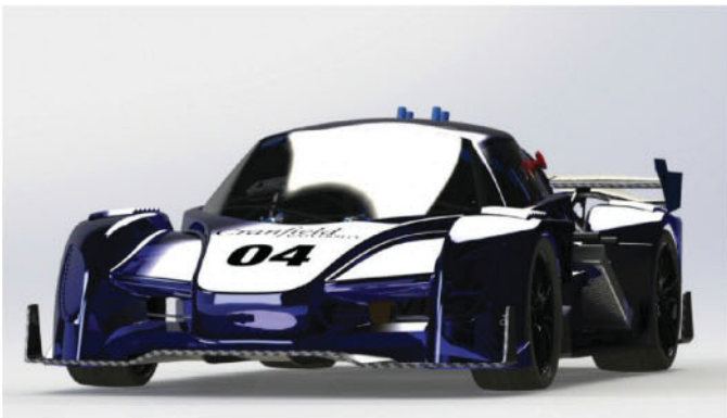
Although the vehicle weight has increased to 1330kg, the power-to-weight ratio is still 24 per cent more than on the base car
