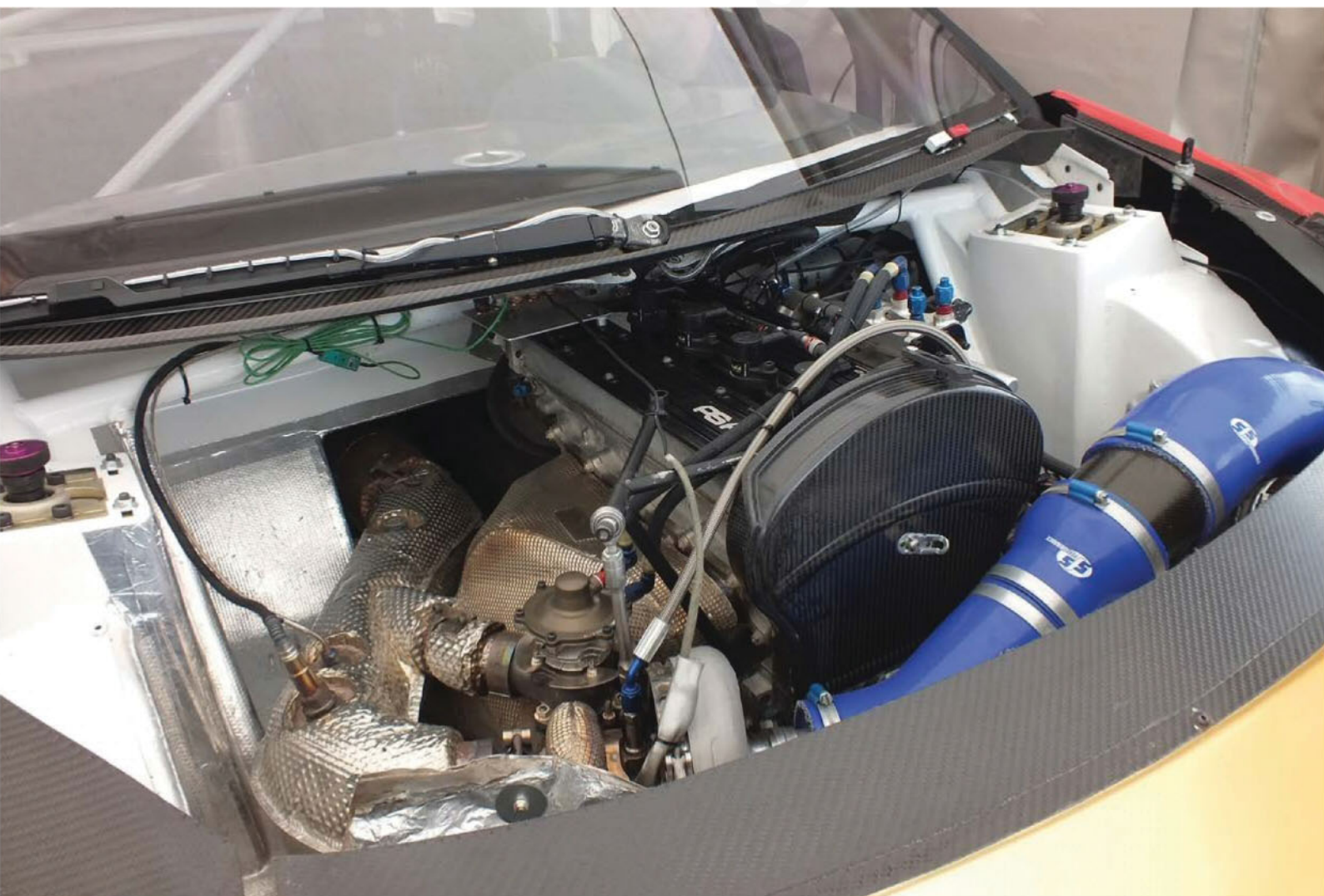
Unlike the LD team cars, Solberg's Citroën DS3s have their engines mounted longitudinally, requiring major surgery to the bulkhead area
