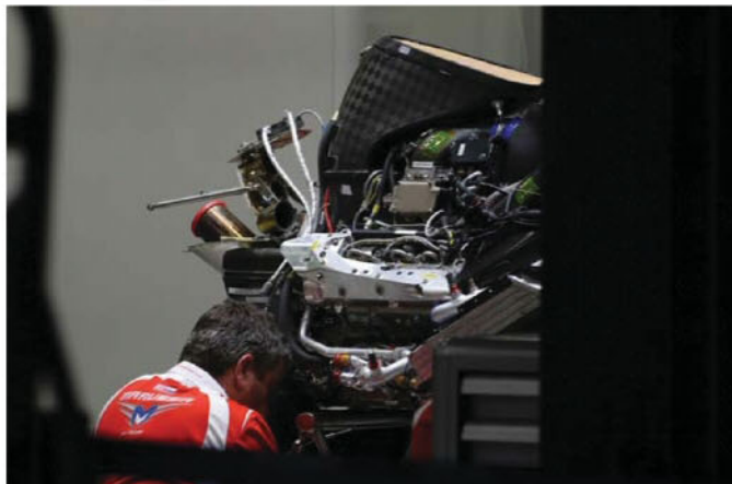
The Ferrari 059/3, 1.6-litre V6 engine, which has a single turbo
