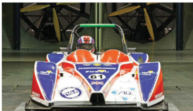
Picture 1: Tiga A's front view highlights its small frontal area. From this angle in particular, the rear wing is almost invisible
