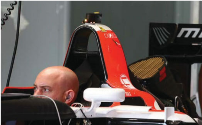
The MR03's roll hoop is the only one on the grid without exposed supports. Instead it features a pair of cooling ducts behind the driver's head
