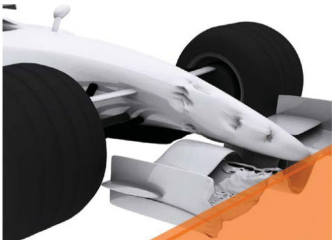
QinetiQ's self-repairing concept suggests that a car would pass through a beam of heat, energising the composite structures to repair themselves
