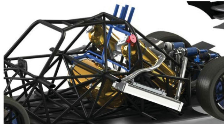
Three hydrogen tanks are mounted in the chassis, the largest in the conventional fuel cell location, while a pair of smaller tanks are mounted on the roll hoop supports. Vent pipes exit on the roof of the car
