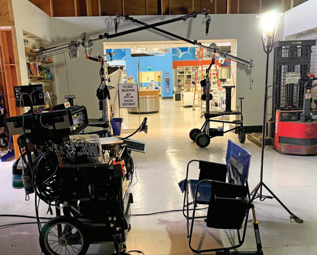
(Clockwise) Darin Knight's sound cart and the two Fisher booms, Steve and Shannon Cain, both booms with offset arms, monitor system, and correct PPE, Steve Cain with an 816 in a blimp, better than a fishpole and a ladder with such a heavy microphone.
