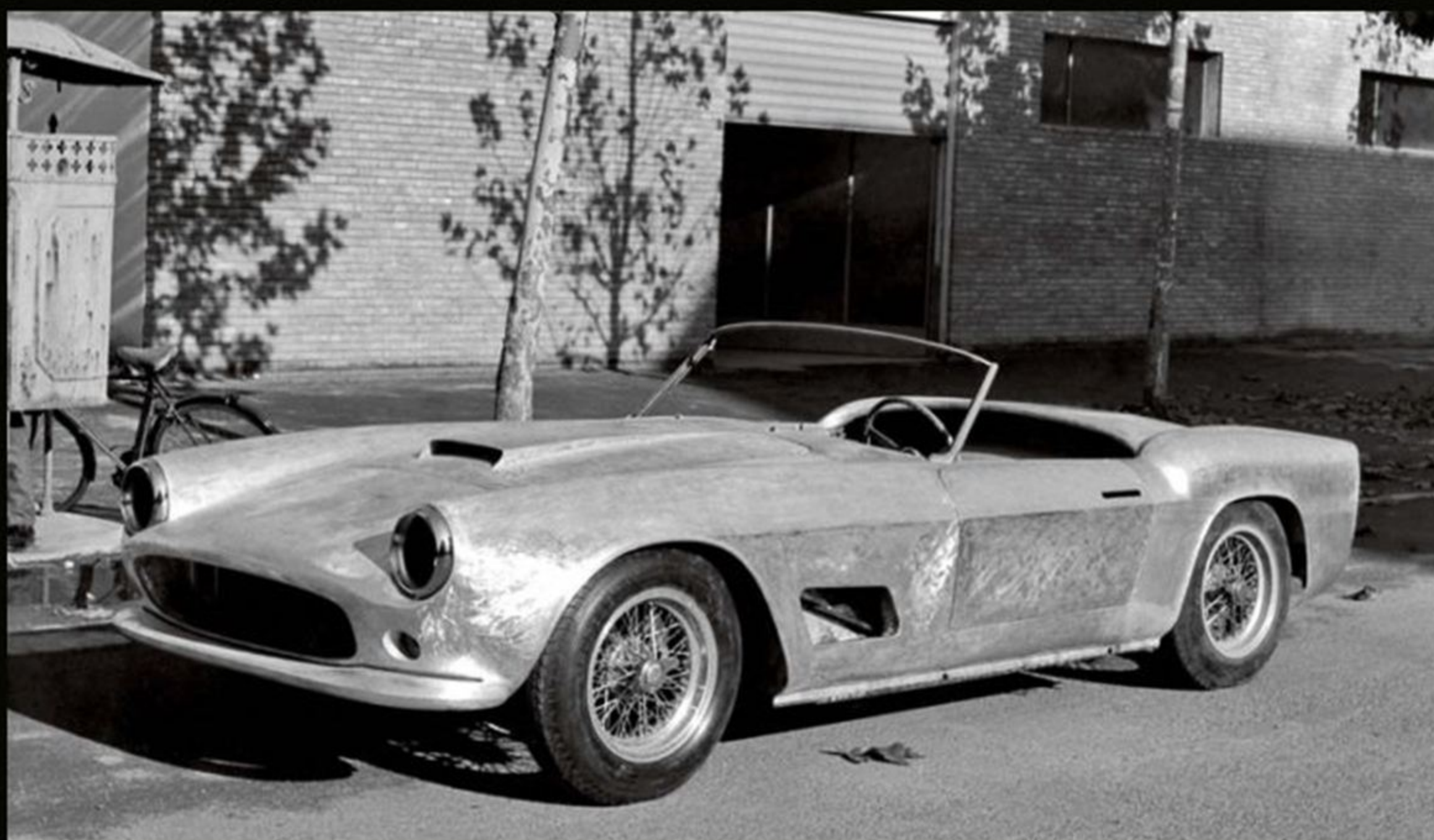
This page – above, the rough body of a 250 California just beaten into shape by Carrozzeria Scaglietti; below, Scaglietti's 166 MM in the 1953 1,000 Miglia, his first Ferrari; bottom, the 250 P, created by Fantuzzi, during a test drive at the Modena Aero-Autodrome
