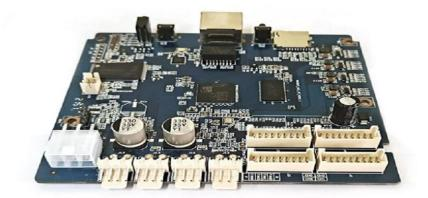
Control boards for mining hardware continue to evolve continuously, as illustrated by the Antminer S19 control board. For miners seeking optimal mining performance, it has advanced features, is compatible with a variety of mining chips, has efficient power management, and has robust cooling mechanisms.
