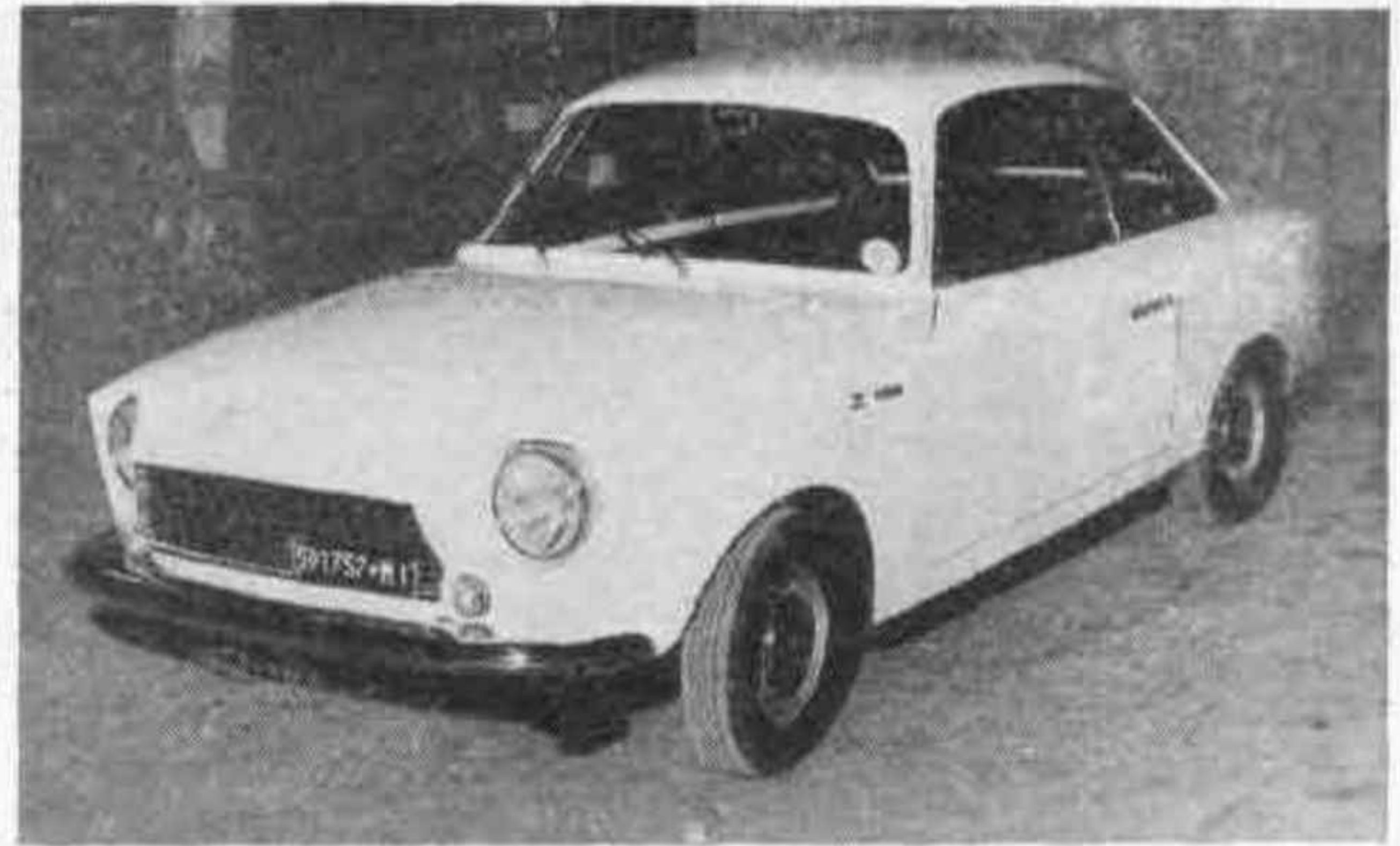
YET ANOTHER MINI VARIATION. —Not only Coopers and Supers and Hornets and Elves but at Earls Court this fibre-glass G.T. coupé by Zagato on a Mini-van base with the "souped up" engine enlarged to 950 c.c.
