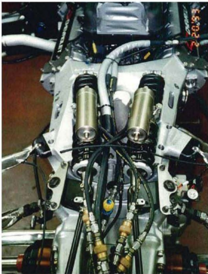
In this pre-installation view, the actuators are at the top, towards the engine
