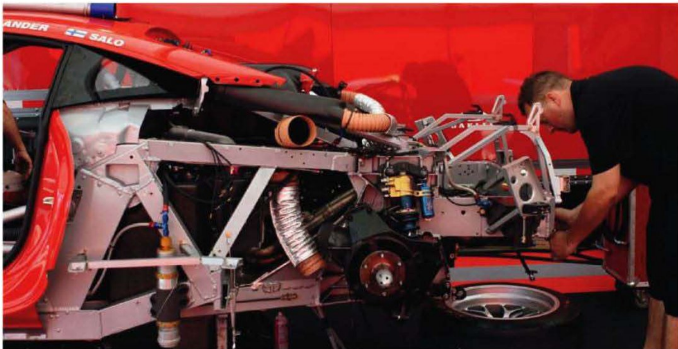
The 458's multi-link suspension underwent the most radical re-design of all, with revised geometry and optimised c of g and polar moment of inertia, making the new car an entirely different handling racecar to the 430 it replaces
