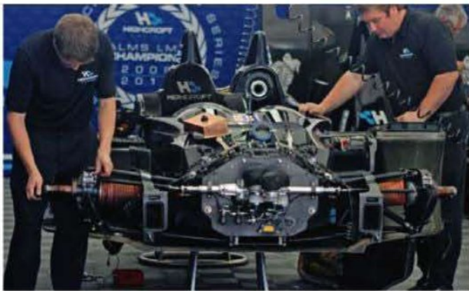
Packaging the wider P1 tyres and wheels, and the associated cooling ducts, presented some issues, but lessons learnt from the P2 project paid off
