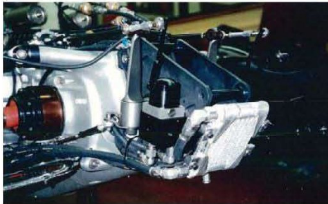
Close up of the left-hand side linkage, showing the hydraulic fluid cooler
