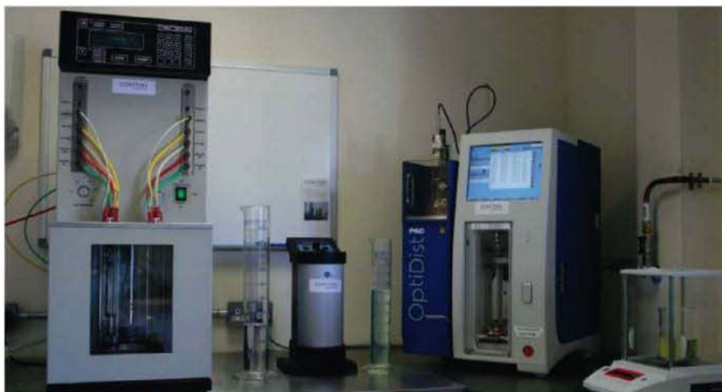
Coryton Advanced Fuels has a range of advance blending equipment including this automated distribution analyzer, used primarily for atmospheric distillation
