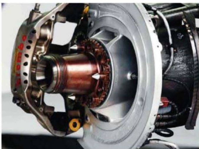
Many Formula One teams use a spline mounting for brake discs which offers reduced weight and mechanical advantage
