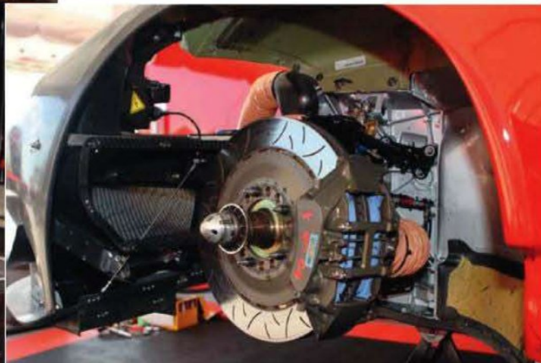
Gone are the production suspension components of the 430, in their place a purpose-designed race set up, with fabricated uprights and control arms
