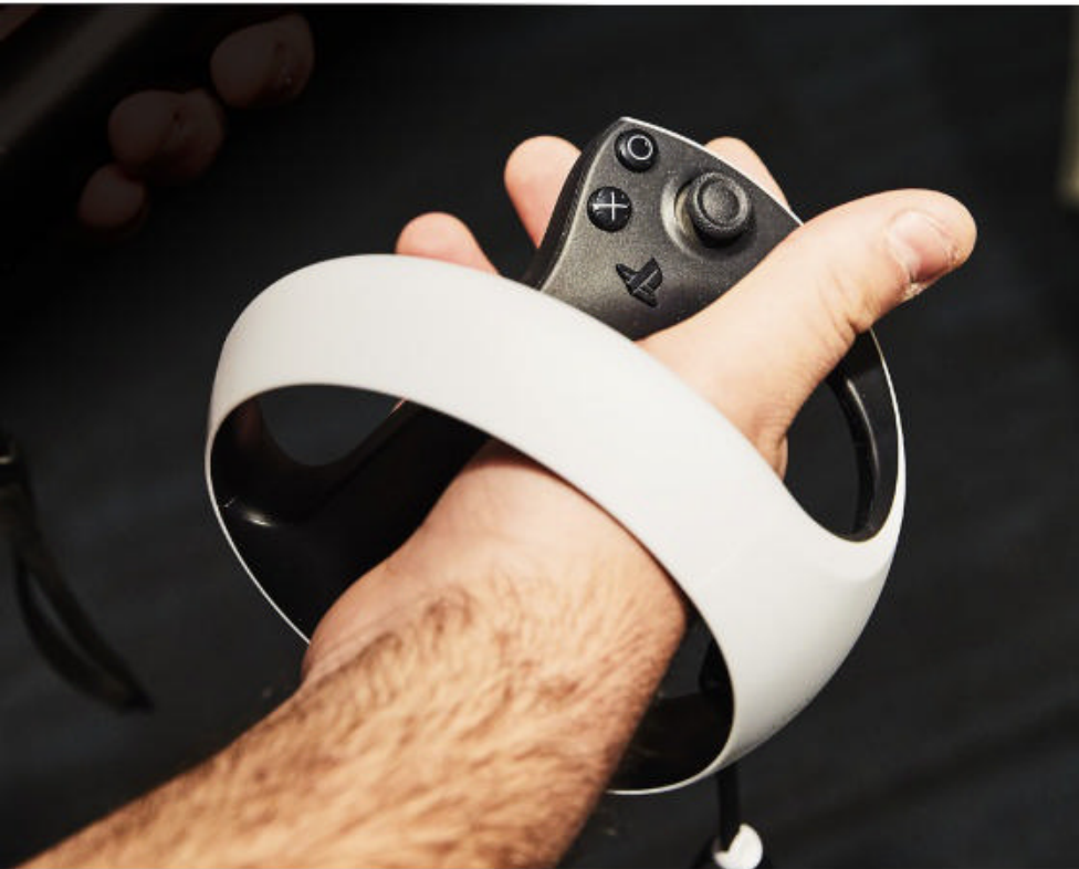
Sony's Sense controller tracks finger movements.
