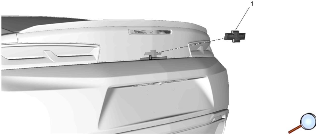
4. Remove existing bowtie (1) utilizing a plastic flat bladed tool. Ensure all adhesive must be removed, otherwise new tape-applied bowtie will not adhere properly.
