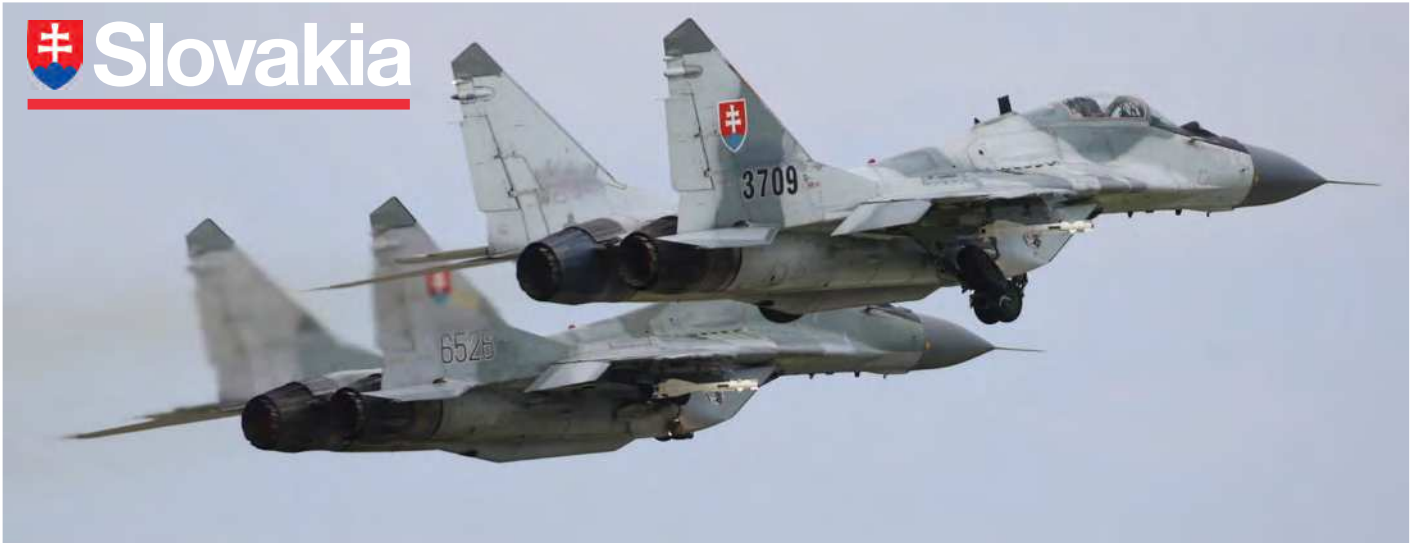
The era of the Slovakian MiG-29 is heading to a close. Here, two single-seat MiG-29AS Fulcrum depart Sliac during a Quick Reaction Alert scramble in September 2018. Note that the aircraft are each equipped with live R-60 (NATO: AA-8 Aphid) short-range air-to-air missiles. All images: Alan Warnes
