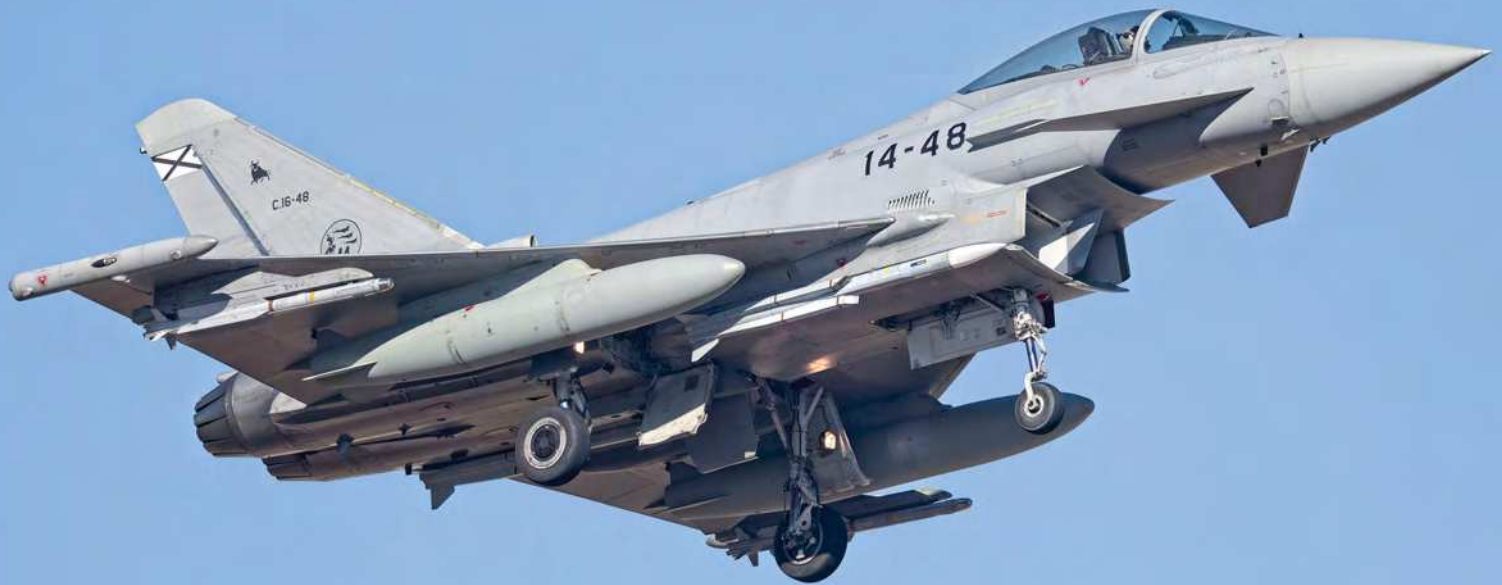
Eurofighters from the EdA's Ala 14 at Albacete-Los Llanos AB were the first to be integrated with MBDA's Meteor BVRAAM. This EF-2000A is equipped with two such missiles on its belly fuselage
