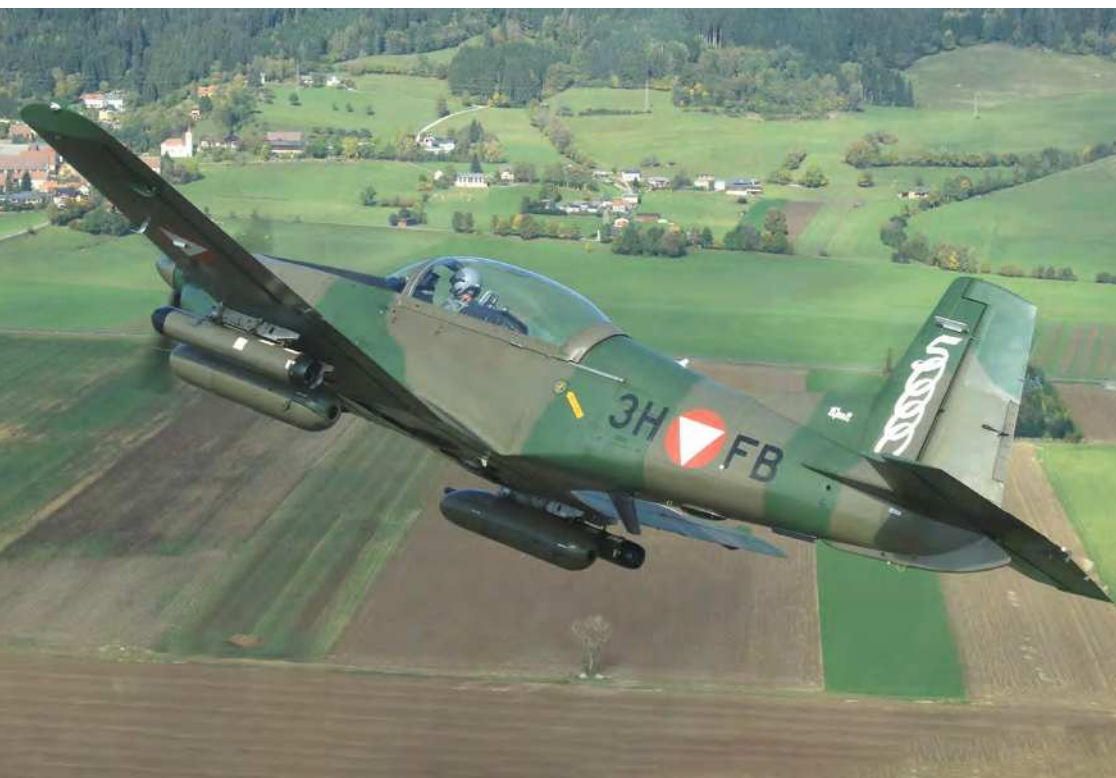
Below: The Pilatus PC-7s are fitted with machine guns and rocket pods for QRA to cover just the 'slow movers', or during times when airspace is temporarily closed for big state-like events Georg Mader
