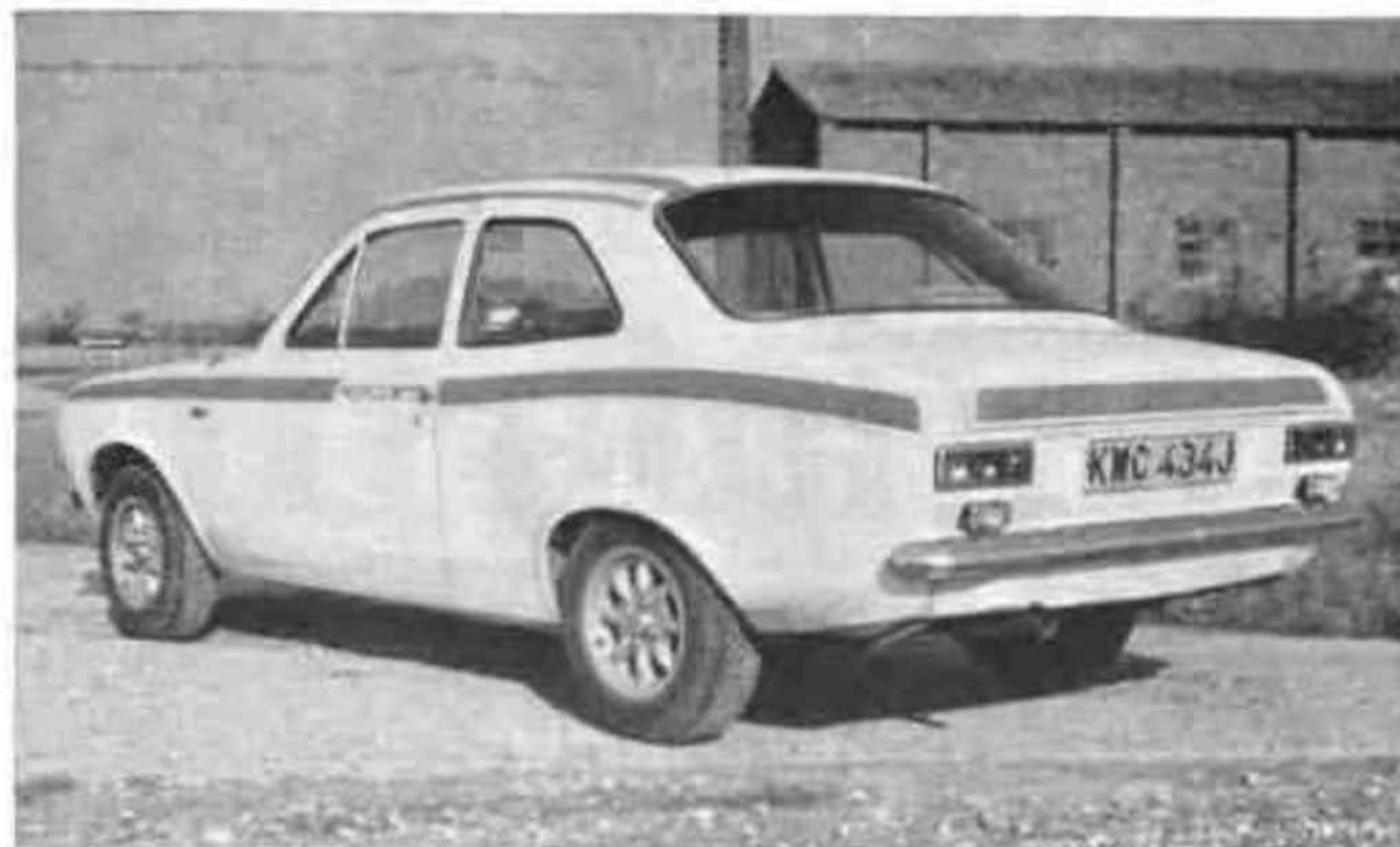
FORD'S Advanced Vehicle Operation is responsible for manufacturing and marketing the Escort Mexico. This latest Escort offers the same mechanical specification as the Escort Twin-Cam and RS 1600 models, but is powered by the much less expensive crossflow 1600 GT unit.
