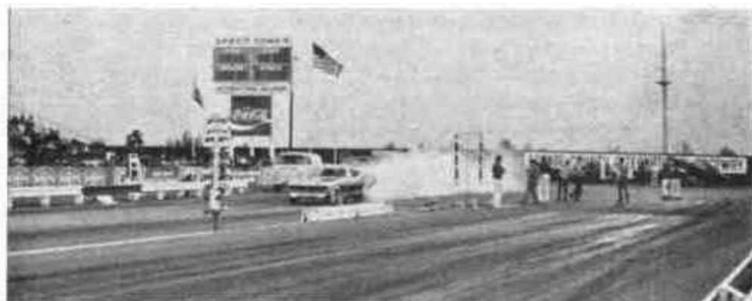
BURNOUT —that's the name given to this smoke-raising operation which burns the track to a suitably gripping surface prior to a timed run. The "Christmas Tree" starting lights can be seen in the foreground.
