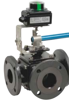
784 - Carbon steel - T port A216WCB body - PTFE seats - Full bore - PS: 16 bar - TS: -20°C/+150°C.
