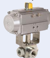
721 ZA - Pneumatic actuated carbon steel ball valve L-port 1.0715 body & ball - TS: -20°C/+100°C.
