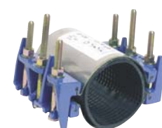
1406 - D Type (2 piece) - 3 bolts x 2 - EPDM - Length 200 mm
