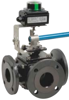
783 - Carbon steel - L port A216WCB body - PTFE seats - Full bore - PS: 16 bar - TS: -20°C/+150°C.
