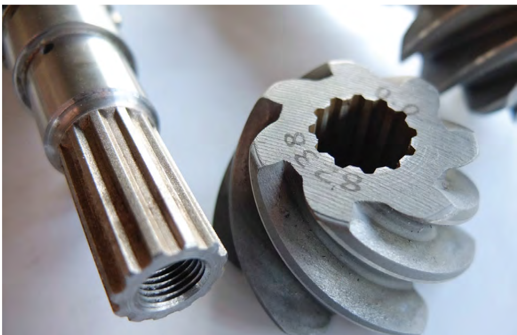
ABOVE The original pinion has been remade with a spark eroded spline
