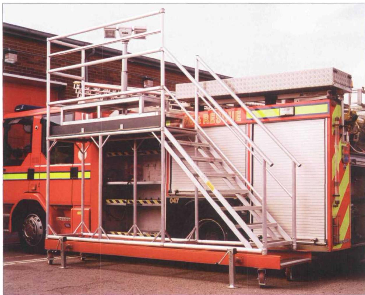
Figure 2.59 Access steps and working platform for vehicle maintenance.
