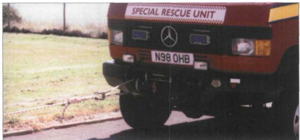
Figure 2.38 Photograph of vehicle being used as a temporary artificial anchor.
