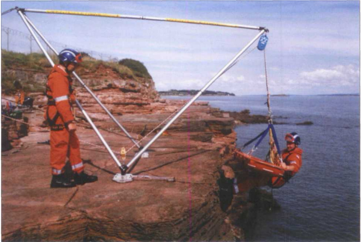
Figure 2.43 Photograph of an artificial high directional (AHD) in use at an edge.
