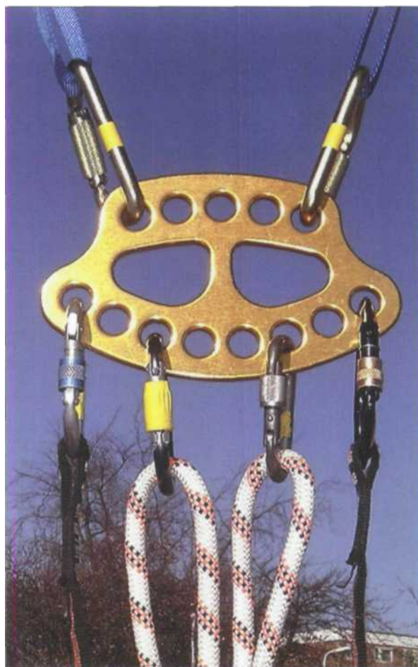
Figure 2.28 Photograph of a rigging plate in use.
