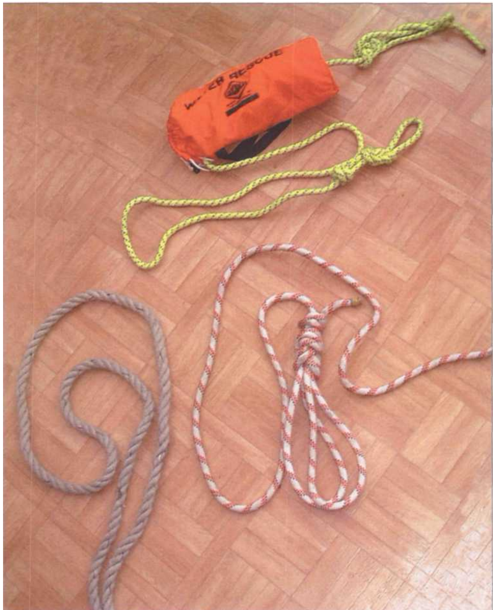
Figure 3.6 Photograph showing a variety of types of rope and cordage including kemmantel rope: British Standard 16mm hawser laid polyester GP line and an example of floating rope.
