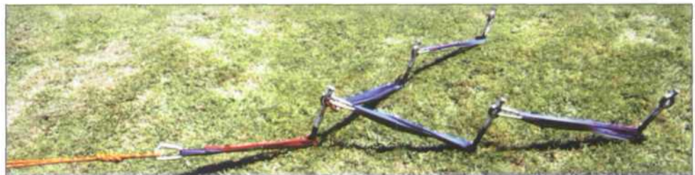
Figure 2.37b Photograph showing V-configuration of ground anchor system.
