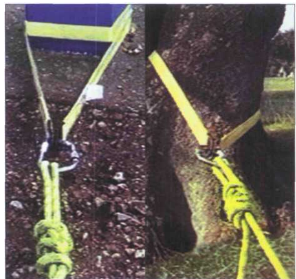
Figure 2.27 Photograph of temporary artificial anchors.
