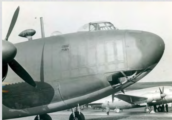
ABOVE Taken during an exhibition at Farnborough in 1945, this image of DW512 shows the type's single-pilot cockpit, which proved controversial during the development phase
