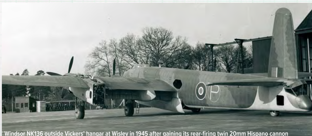
Windsor NK136 outside Vickers' hangar at Wisley in 1945 after gaining its rear-firing twin 20mm Hispano cannon
