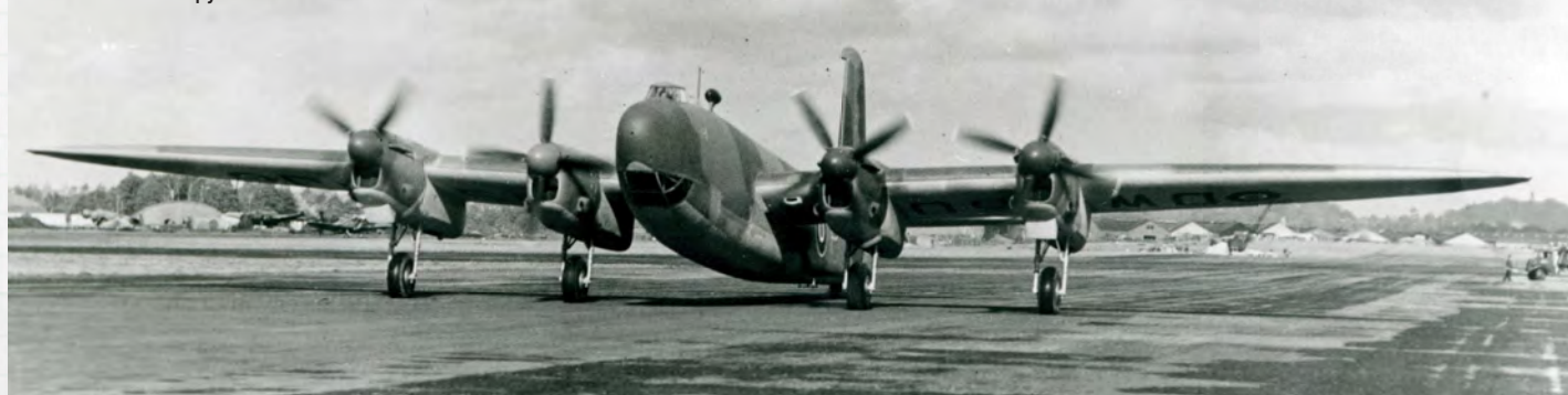
BELOW Vickers Windsor DW506 running on the runway at Farnborough in 1943 showing the type's evident wing droop and fighter-style canopy
