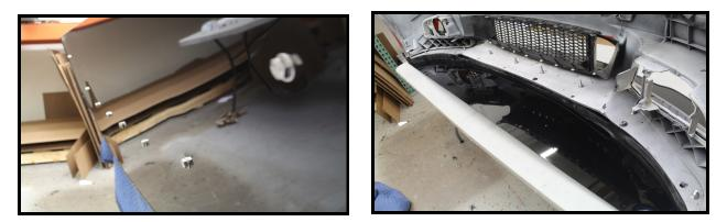
10. FINAL-TEST. Push down on splitter to make sure all bolts will hold up and there is no flair in the splitter.
