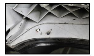
6. Once the bolt is fully through the hole, add another washer On the inside of the bumper, then place the locking nut onto The bolt (hand-tighten till you can no longer tighten the nut).
