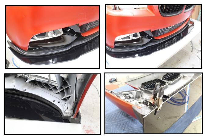
4. Using a 1/4 drill bit prepare to drill through the splitter all the way through the bumper. Repeat process till all holes drilled. \*MAKE SURE BOLTS ARE AS FAR IN TOWARDS THE FRONT OF THE BUMPER AS POSSIBLE.\*
