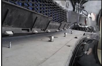
8. Once all bolts are in place, double-check to make sure The splitter is flush with the bumper. Then, if everything Looks good, begin to tighten the locking nut.
