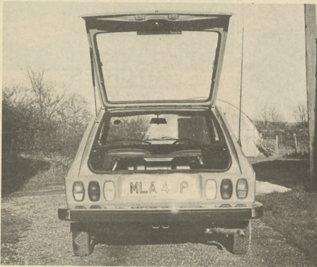
A high rear sill necessitates the expenditure of much effort in loading luggage or assisting elderly dogs.
