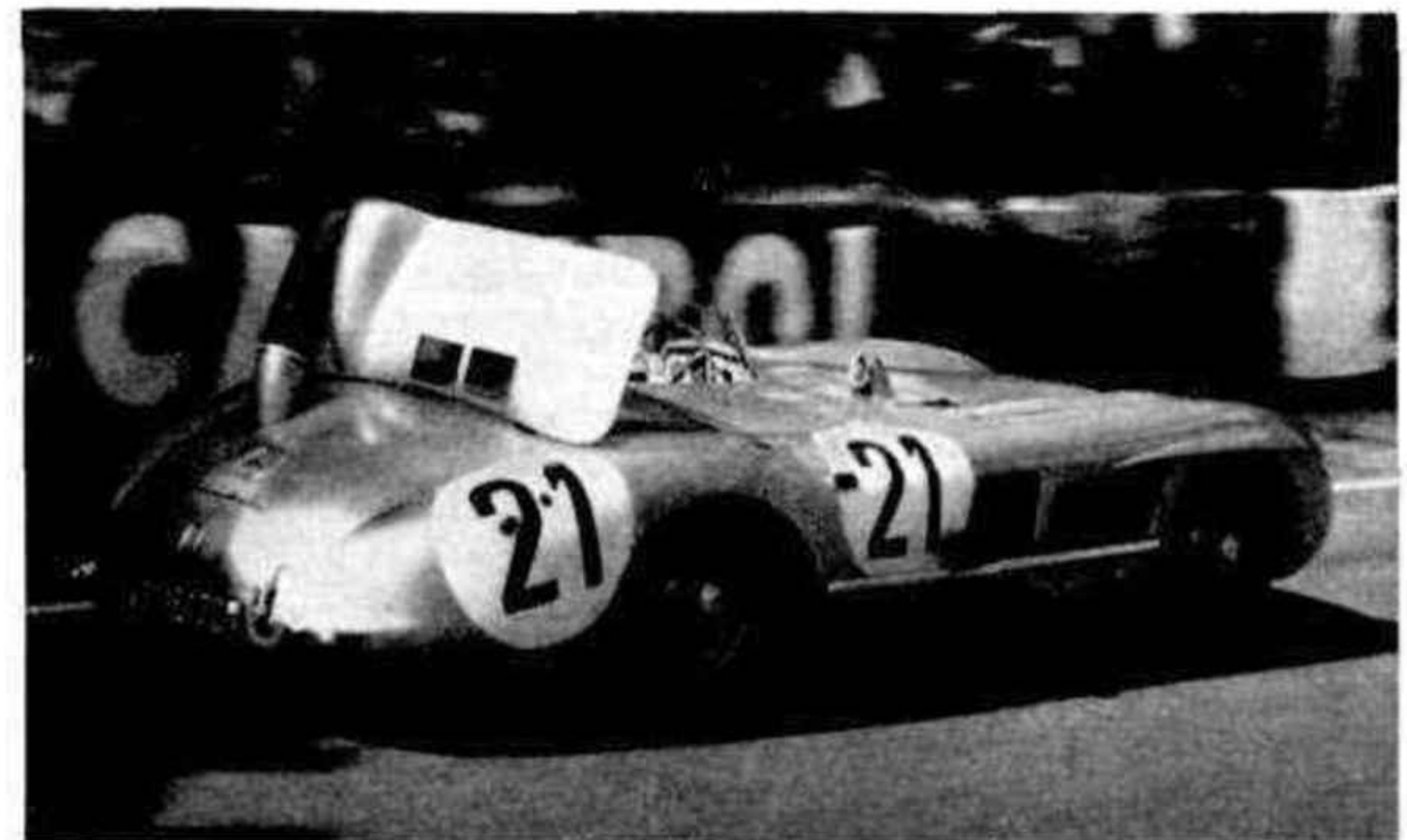
"BUILT-IN HEADWIND."—The hydraulically-operated air-brake of the Mercedes-Benz at Le Mans was most effective. Kling is seen slowing down for Tertre Rouge corner. The tall fuel filler is visible as are the two windows to give vision for the rear-view mirror. On the side of the body by the forward number can be seen the coloured identification light used by the team
