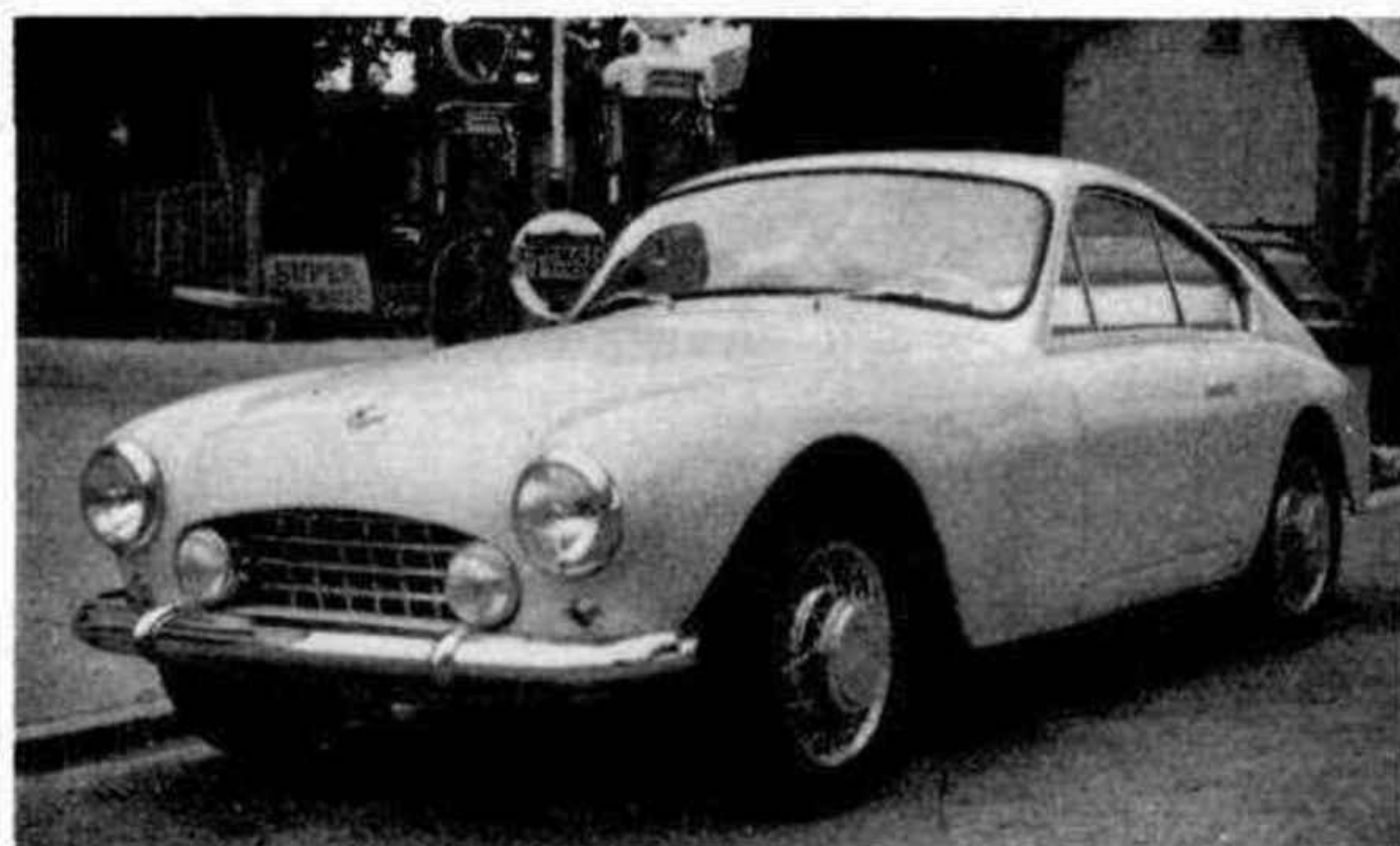
SPECIAL CITROËN. —The special coupe constructed by the proprietor of the B.P. garage in Albi, as described in the text. Using Light Fifteen Citroën front suspension, drive and power unit, the resulting Gran Turismo coupe proved a rapid, if somewhat harsh, motor car in the best Italian tradition.
