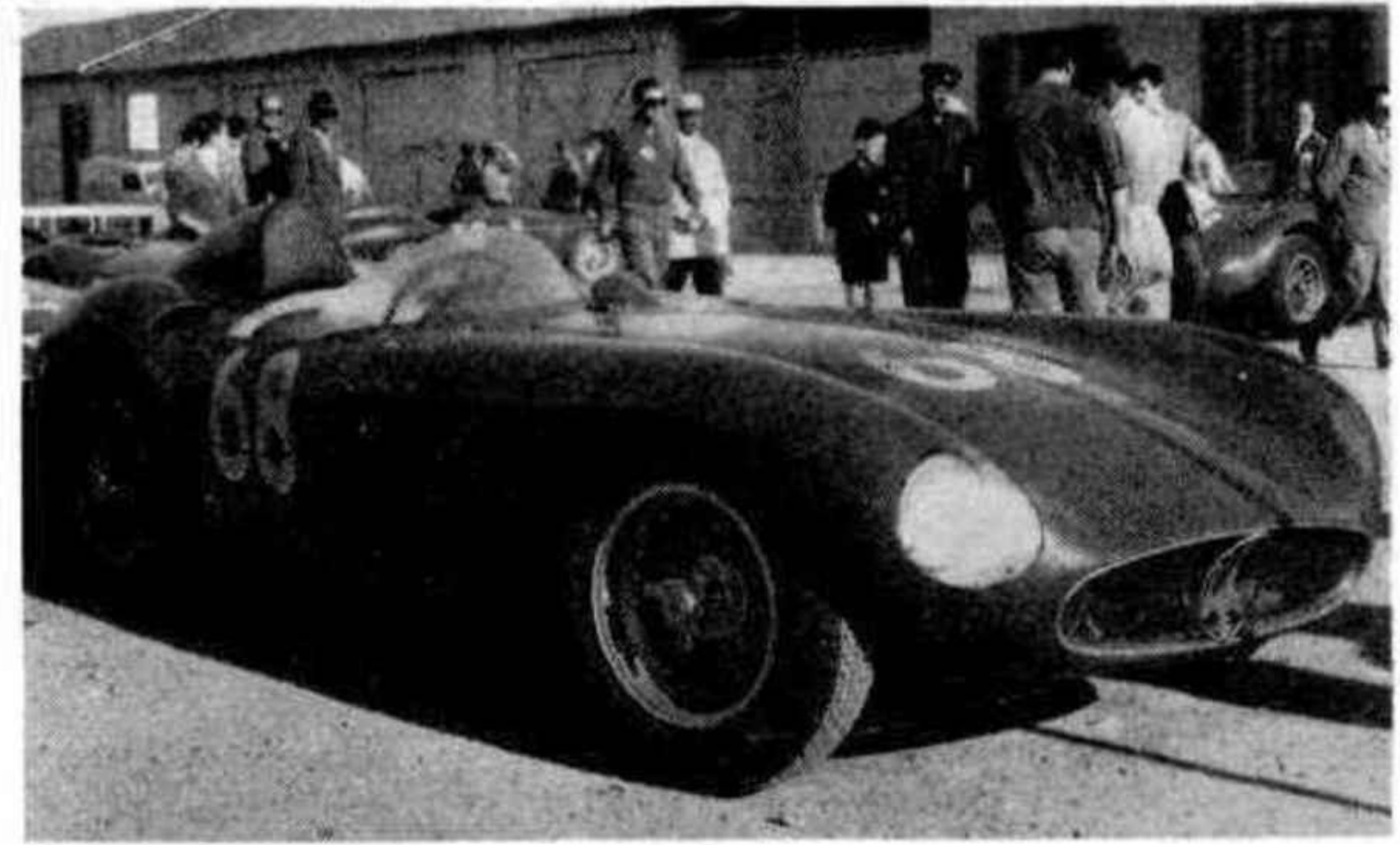
MODERN 3-LITRE. —The six-cylinder 3-litre sports Maserati, with which Behra and Musso won the Supercortemaggiore race at Monza, is developed directly from the Formula I Grand Prix car. The general likeness to the smaller 2-litre sports car is clearly seen, though these 3-litre models have right-hand steering and a headrest.
