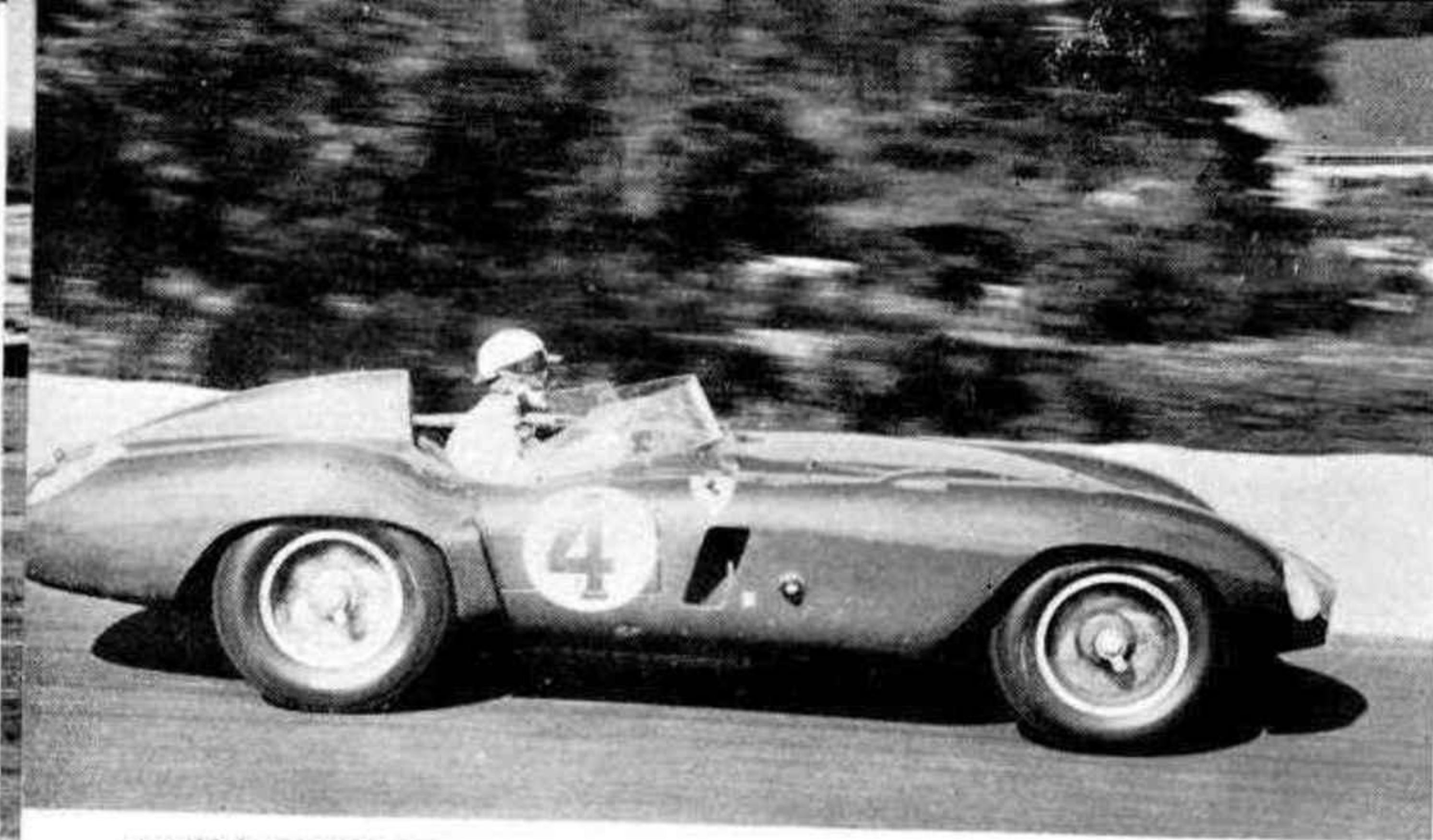
SLEEK MONSTER. —Castellotti at speed in his 4.4-litre Ferrari 6-cylinder on the Mulsanne straight, showing off the nice lines of the Scaglietti-built body. In front of the rear wheel is an air scoop for the tyres and in front of that a large under-bonnet air exit.
