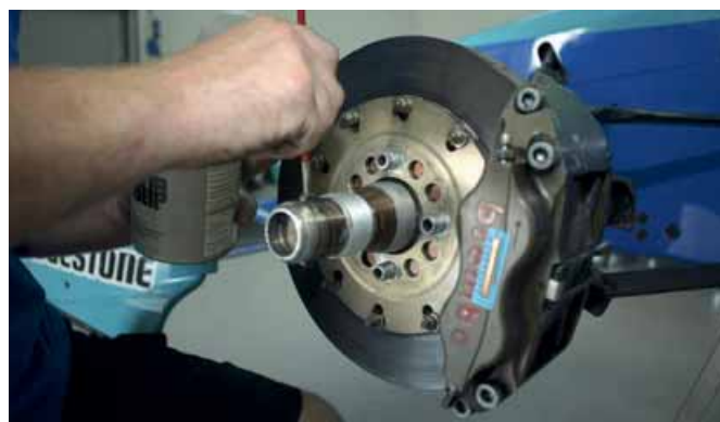
Original brakes were unsatisfactory, so were changed to Brembo for race two
