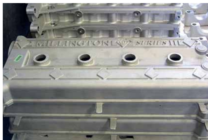
The build process starts with the X-rayed, certified castings
