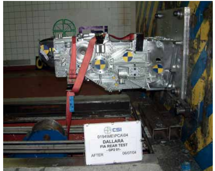
Nosecone and gearbox undergoing crash testing at CSI. After initial reliability problems, Mecachrome gearbox is now sorted, though is still considered too heavy
