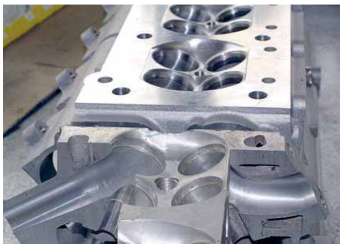
In the foreground is a section through a YB cylinder head, behind is Millington's new head, with shallower valve angle, and different port face angles. Just visible on the inlet side (left) is the barrel throttle option
