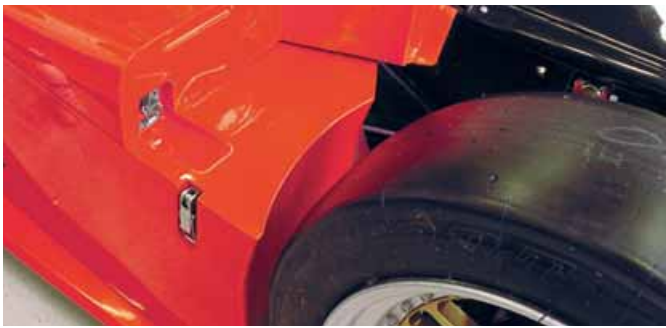
Left and right: more over-centre catches from Protex. Its fasteners are available in different strengths depending on application
