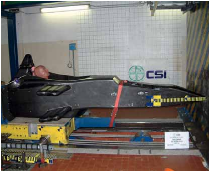
Nosecone and gearbox undergoing crash testing at CSI. After initial reliability problems, Mecachrome gearbox is now sorted, though is still considered too heavy
