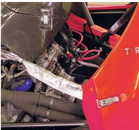
Left and right: more over-centre catches from Protex. Its fasteners are available in different strengths depending on application
