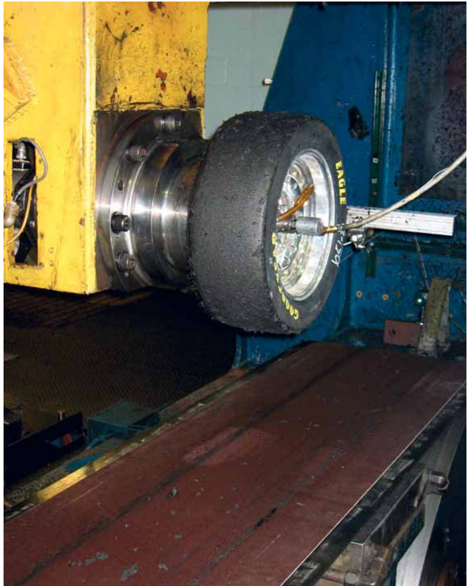
One of the Goodyear Formula SAE tyres on the tyre test machine, post-test. Note the build-up on the tyre
