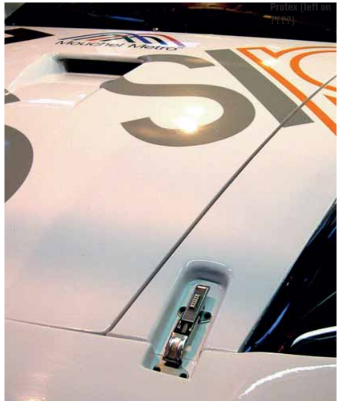
Left and right: more over-centre catches from Protex. Its fasteners are available in different strengths depending on application
