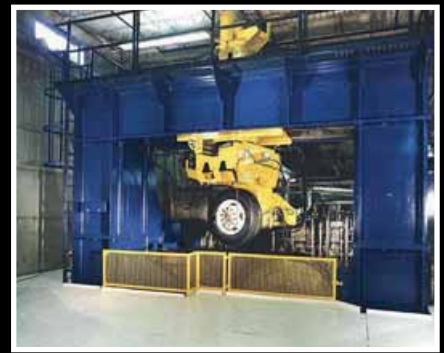
The Calspan Tyre Research Facility tyre tester
