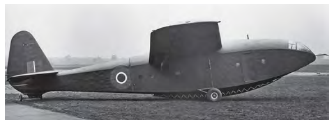
Hengist prototype DG573 during trials in October 1942, showing the under-fuselage rubber air bag provided to help the airframe take the loads experienced on landing at high weights. ALAMY
