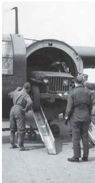
ABOVE: Civilian workers with a newly delivered, still disassembled Horsa at Brize Norton. KEY COLLECTION ABOVE RIGHT: The Horsa II introduced a hinged nose, rendering the loading and unloading of cargoes such as Jeeps easier. KEY COLLECTION
