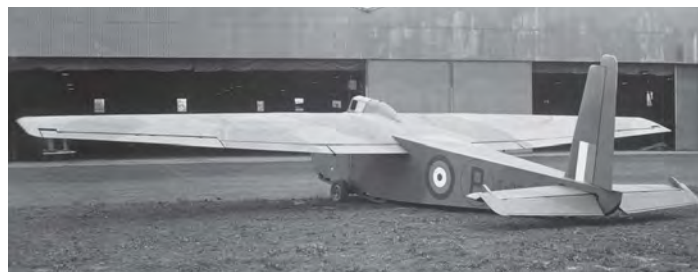
The GAL50 was a half-scale prototype of the Hamilcar. Serial T-0227 crashed at the end of its maiden flight in September 1941. KEY COLLECTION
