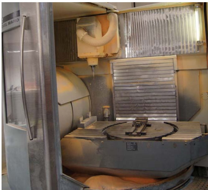
Every NC program has to pass through VERICUT to ensure the safety of the machine tools. VERICUT supports Freeform Technology's production of complex moulds and composite patterns for the motorsport sector
