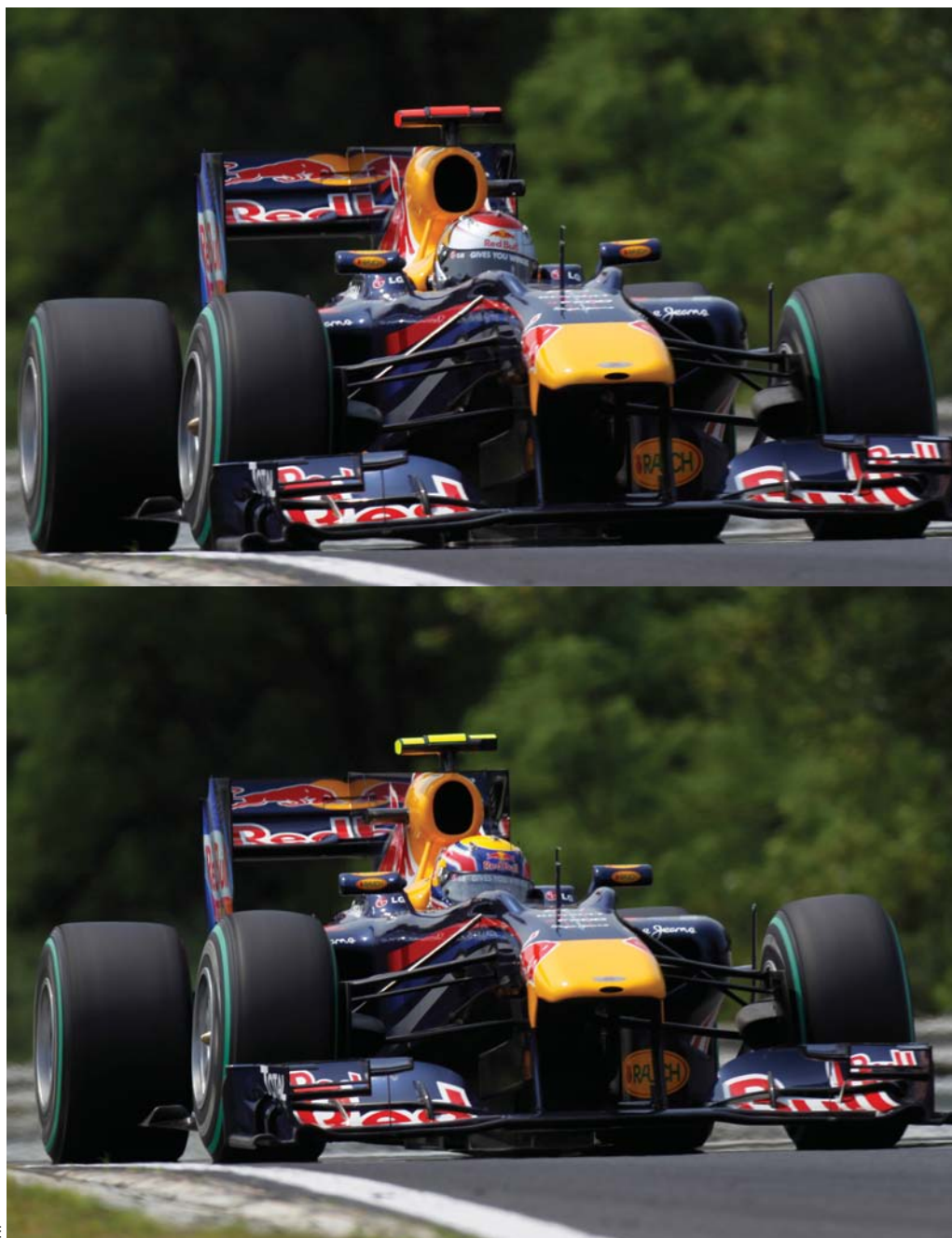
The flexible front wings caught on camera during the 2010 Hungarian Grand Prix: the front of Sebastian Vettel's RB6 (top) hugs the ground, while Mark Webber's (above) is in flex
