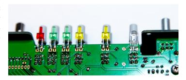
After soldering all LEDs tot the Mainboard unscrew the Frontpanel again. Put the 25mm Spacers on the Mainboard and add the LED-Meter Board. Use the screws to secure the LED-Meter Board. Put the Frontpanel back on again and tighten the Nuts to the bracket. Now we will finally solder the remaining legs of the Pots as they should be perfectly centered now.
