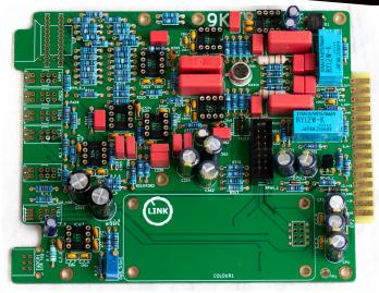
On the LED Meter Board we also add the electrolytics and Wima Capacitors and Board connections, and cut leads after soldering as short as possible. We will do this process later with Potentiometers also, since we need to make sure that this Preamp doesn't touch any neighbour modules of any kind.
