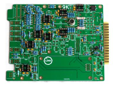
Continue on the LED Meter Board and add all Sockets. Normally we solder first one pin in and trim all of the other Pins as short as possible and continue after that with soldering all other pins on that Board.
