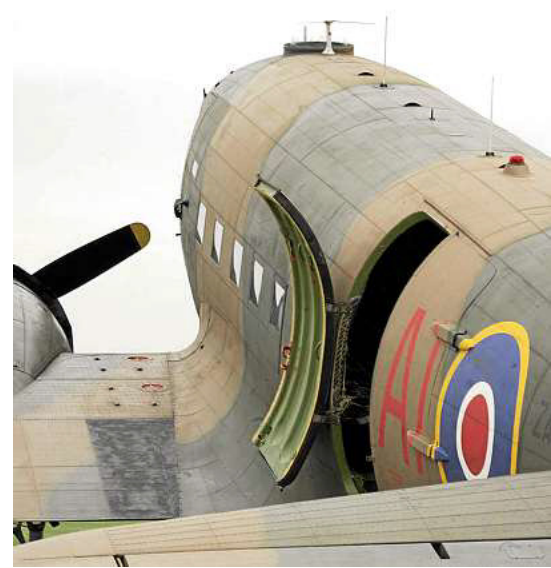
The large rear cargo door was one of the reasons for selecting the Dakota for Operation Wildhorn. Julian Humphries
