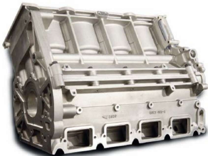
The MT1 block was cast by Zeus, now part of Caparo. Note the inclined layout
