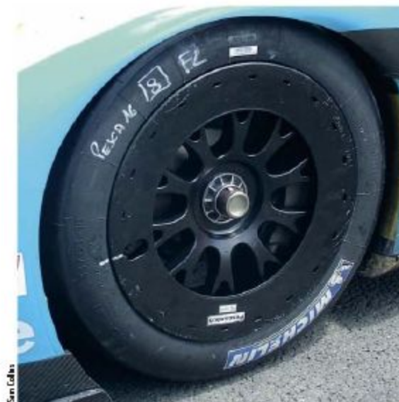
Pescarolo fitted these controversial semi rim blanked wheels to its works LMP1. Porsche had previously not been allowed similar items
