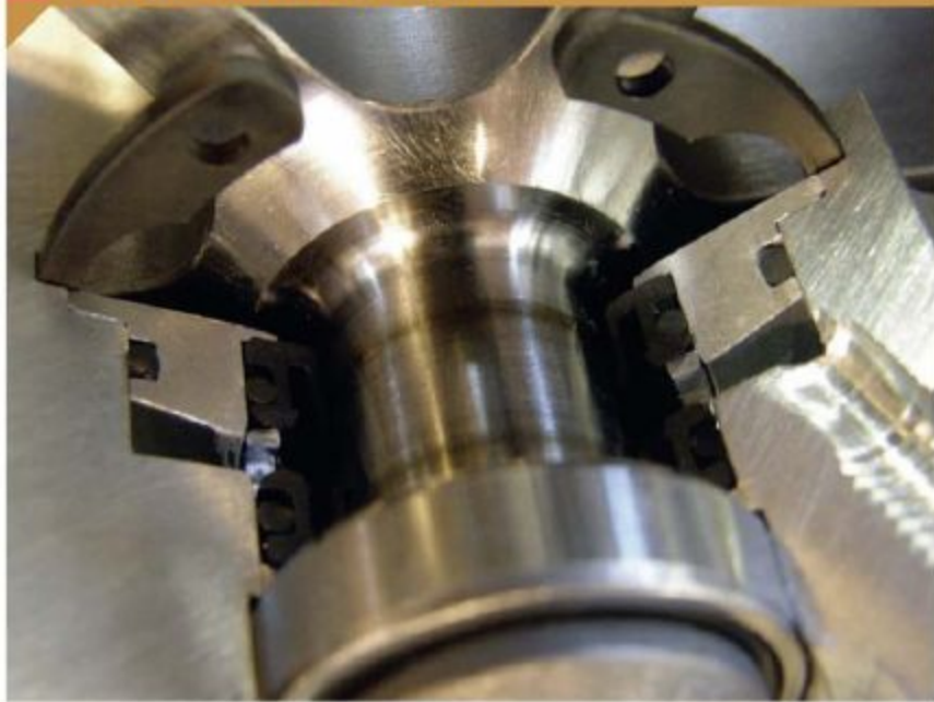
The twin lip shaft seal capable of maintaining a vacuum on the Flybrid KERS unit
