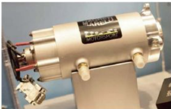
The Magneti Marelli motor / generator unit
