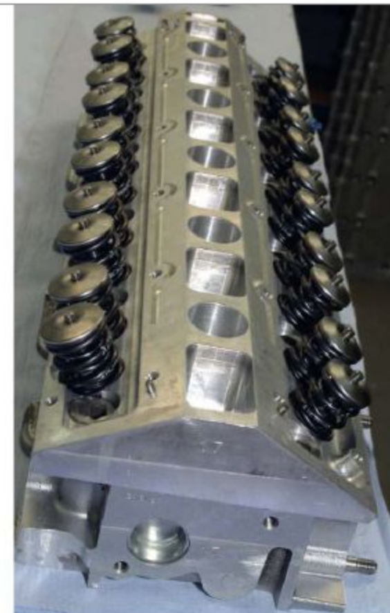
Valve angles and inlet port positions had to remain as standard measured from specific reference points, opening the door wide to interpretation
