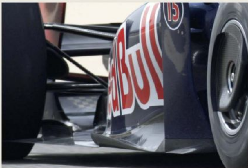
The main reason Red Bull has used pull-rod suspension this year is due to changes in the 2009 F1 aero regulations
