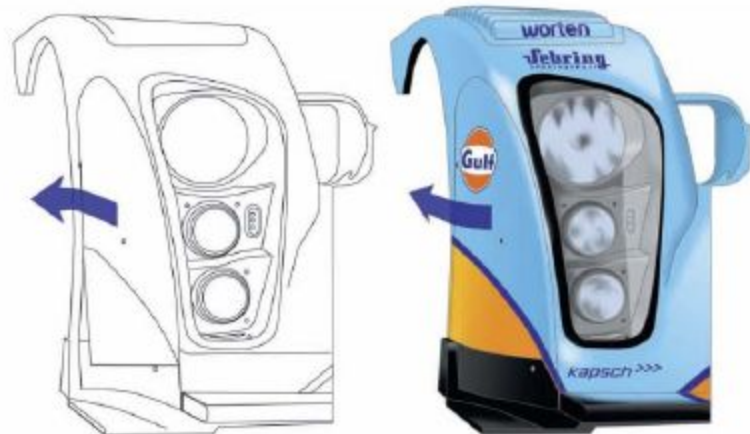
Prodrive modified the front of its Lola B08/60s in an attempt to reduce drag, the concave panel where it usually has dive planes mounted (above left) being replaced with a smooth, convex part
