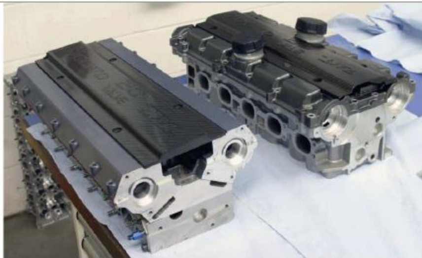
The Super Touring rules said nothing about the angle the head had to sit on the block - a loophole TWR exploited to great effect. The standard Volvo head is on the right in this photo, the fully compliant TWR version on the left
