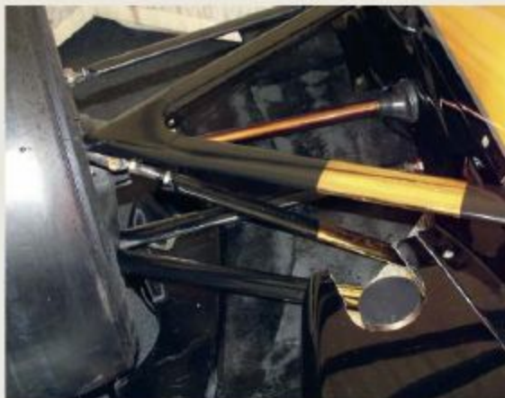
Mygale uses pull rod rear suspension on its Formula 3 design
