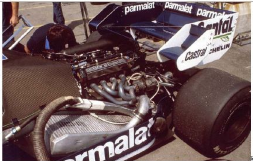
The M12/13 engine in the Brabham BT53 of 1984 produced 880bhp in race trim but much more in qualifying
