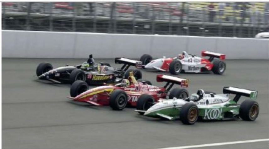
With the Handford wing fitted CART racers of the past were seeing speeds of 240-250mph on the ovals. According to Robertson, this was too high. He believes a sensible speed for Indy Cars is something in the high 220mph range
