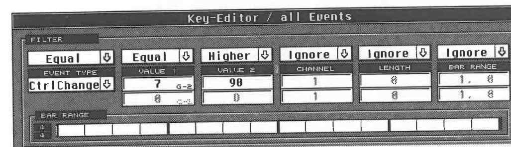
All MIDI Control Change number 7 (volume) events with a value greater than 90.
