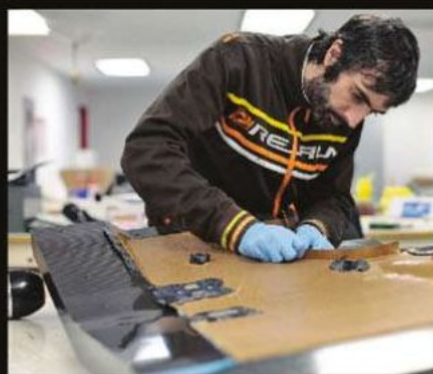
The, er, hairdryer The best way to cure parts, without them bubbling due to excess heat, is with a standard hairdryer
