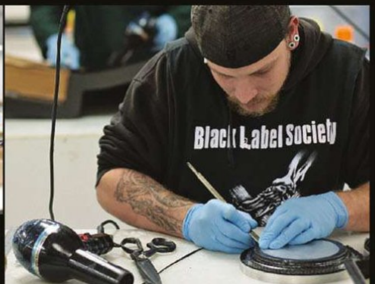
The, er, hairdryer The best way to cure parts, without them bubbling due to excess heat, is with a standard hairdryer
