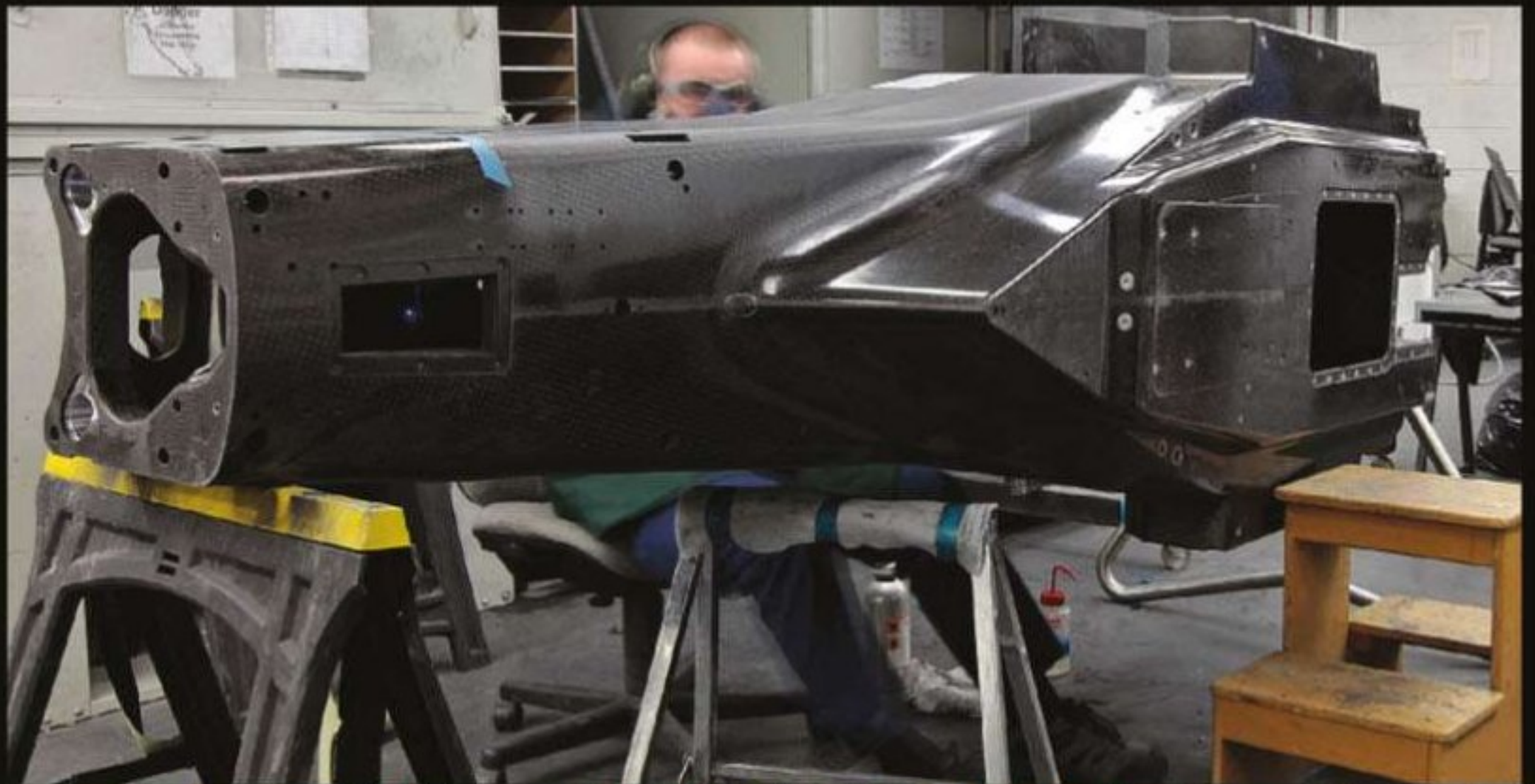
The tub Also known among the team as the 'driver box', the tub is the first thing to be designed and made in the process of building a new F1 car. Caterham's 2012 version was signed off before the August shutdown
