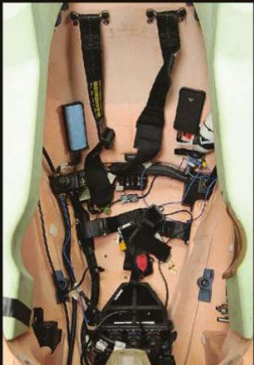
The full-scale replica Made by rapid prototyping, this model allows the team to map out all of the car's internals
