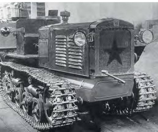
BELOW: STZ developed a military version of the STZ-3, with significant modifications, an open cab for maximum military driver comfort and road tracks. This is the prototype as completed at STZ
