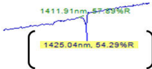
Figure 14.7 Spectrometer readings for %R vs. wavelength for BD-RE disc for egg white.
