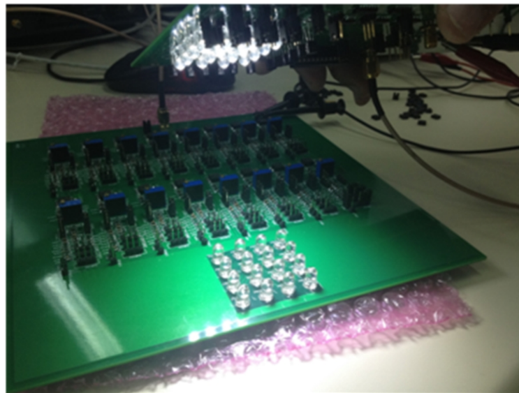
Figure 10.8 Photo of the 16-channel VLC receiver (top left) and transmitter (top right).
