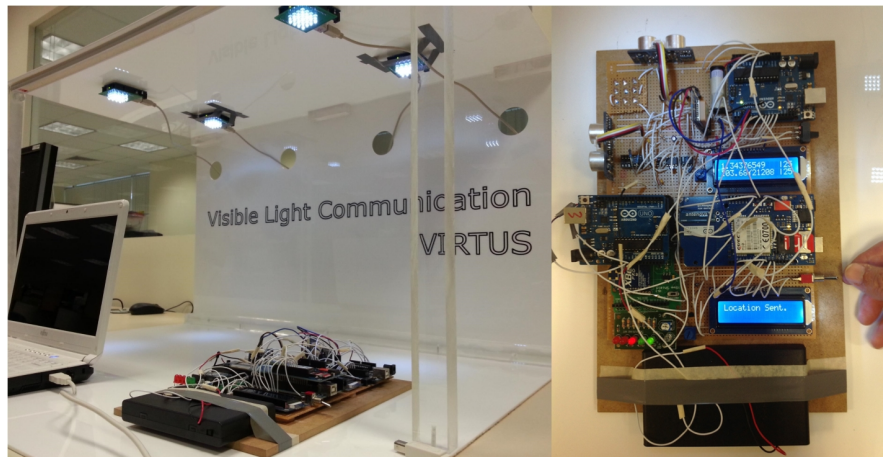
Figure 12.1 VLIPS (Visible Light Indoor Positioning System) prototype: receiver device and 4 LED transmitters.
