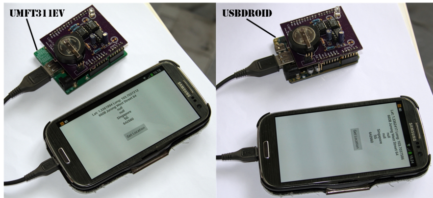
Figure 10.18 Version 2 transceiver with the initial app: (left) UMFT311EV's pinout is slightly different from Arduino's pin layout. The TX and RX pins have to switch position; (right) USBDR0ID has no such problem. The Version 3 pcb design is an improved version made to accommodate both bridge modules.
