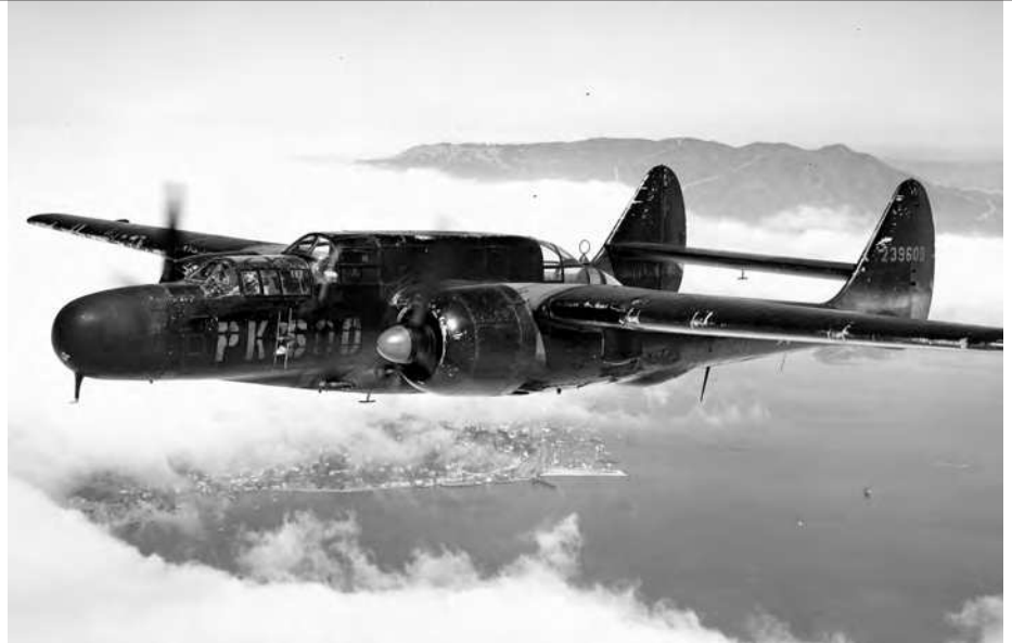
ABOVE: The Northrop P-61 Black Widow was the first aircraft designed with an integral nose-mounted radar that made it an excellent night fighter. OPPOSITE: New B-25 Mitchell bombers undergo final inspection at North American Aviation's manufacturing plant at Inglewood, California; the company produced 26,000 B-25s. American industrial capacity and achievement overwhelmed the enemy.
