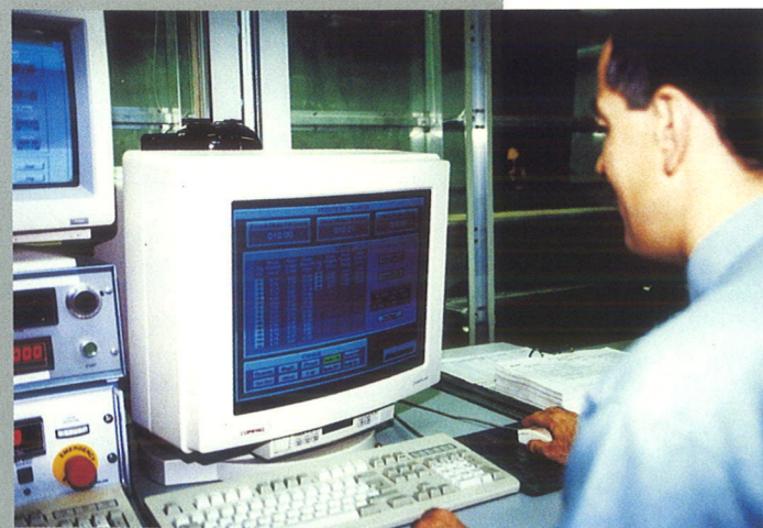
All wind tunnel functions are computer controlled. McLaren's data acquisition system extracts every conceivable force applied in every direction. The measurements are taken from a precise electronic balance located in the car
