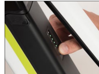
Check the state of charge
