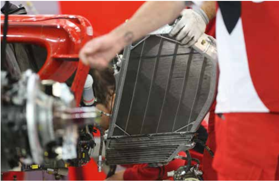
A 2014 DF1 engine needs to reject around 113kW of heat from the water radiator and 58kW from the oil radiator
