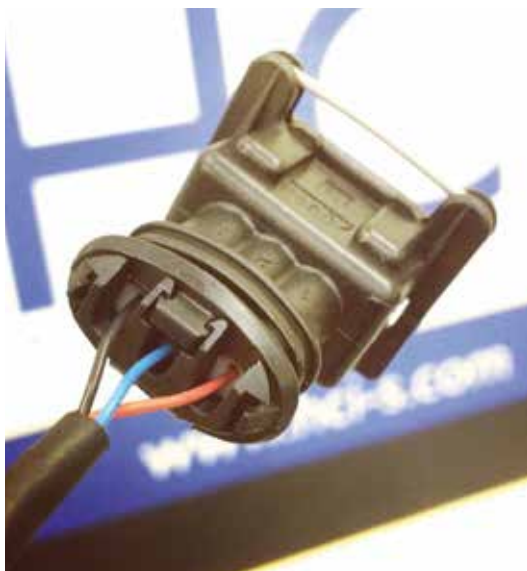
A connector showing the power, signal and ground wires
