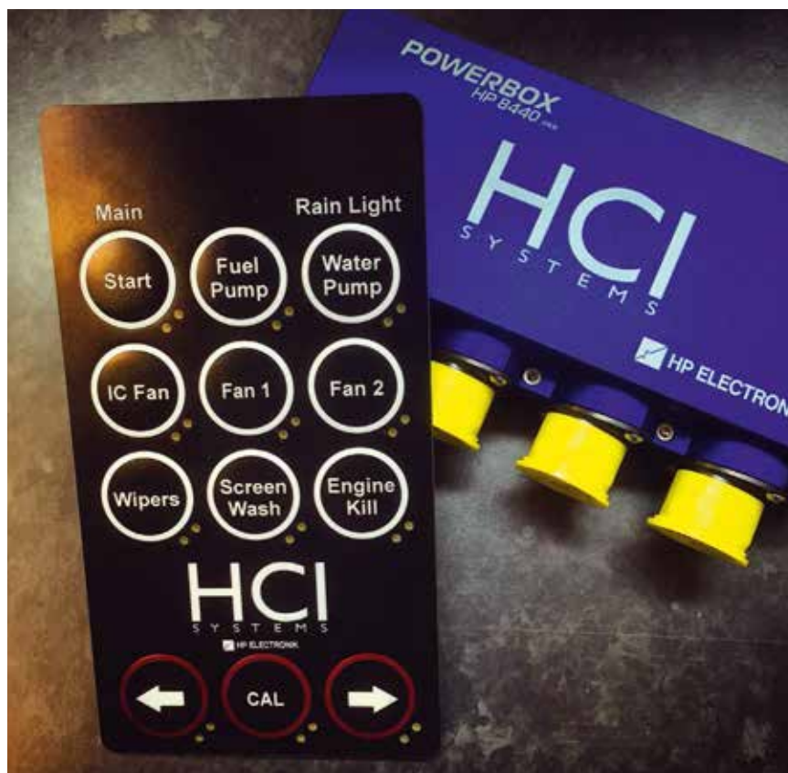
The HP8440 Powerbox from HCl Systems replaces traditional fuses and relays by controlling all the power
