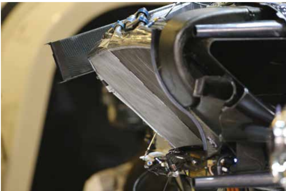
McLaren 2014 right hand side cooler arrangement unclothed showing two different types of heat exchanger
