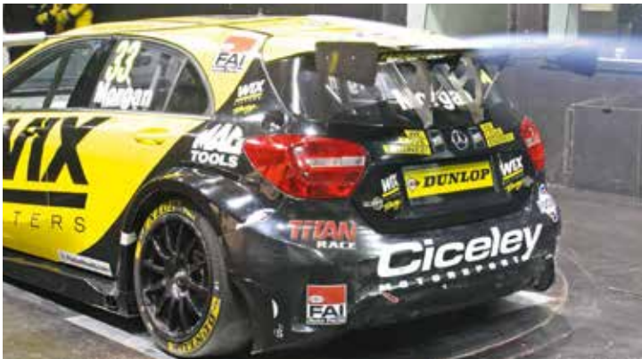
Photo 4: The smoke plume within the wake shows how close the wing is to the wake itself
