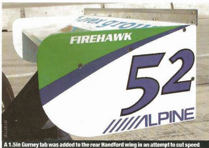
A 1.5in Gurney tab was added to the rear Handford wing in an attempt to cut speed
