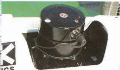
Pop-off valves were set to further cut boost
