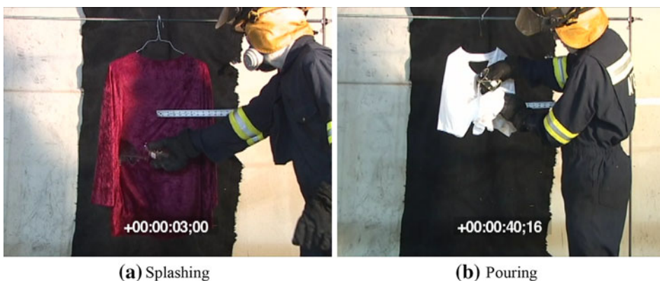
Figure 4. Gasoline was applied to the clothing via (a) splashing and (b) pouring.
