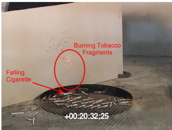
Figure 2. Burning tobacco fragments created by striking a solid surface.
