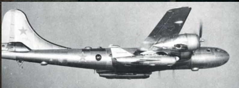
The prototype of the Tu-4K cruise missile carrier with piloted KS-1 missile prototypes during tests.
