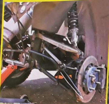
The rear suspension with double wishbones.
