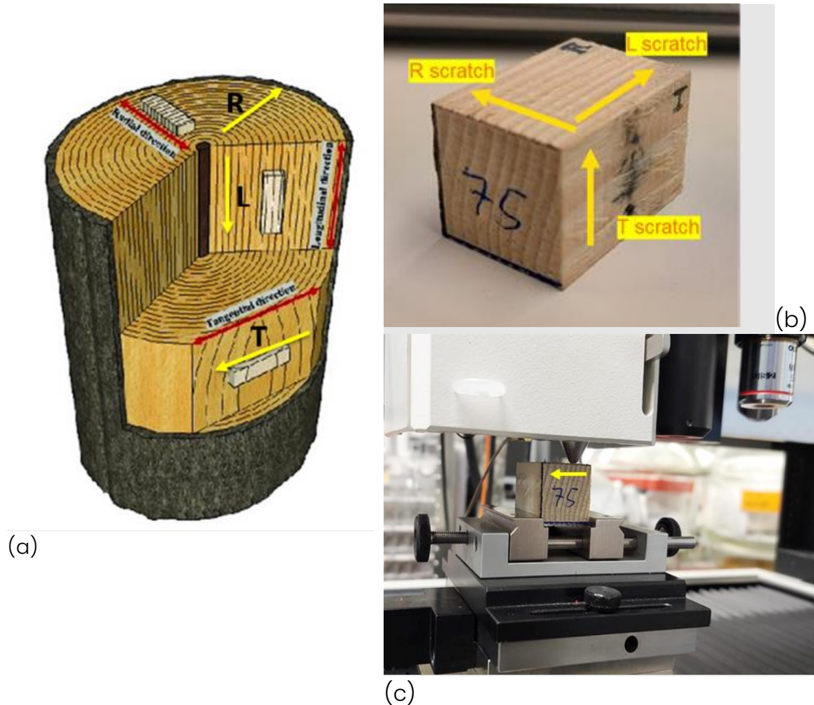
Figure 15 (a) and (b) The scratch directions R, T and L of the wood sample. (c) The test sample in the Micro-Combi tester positioned for scratch testing.
