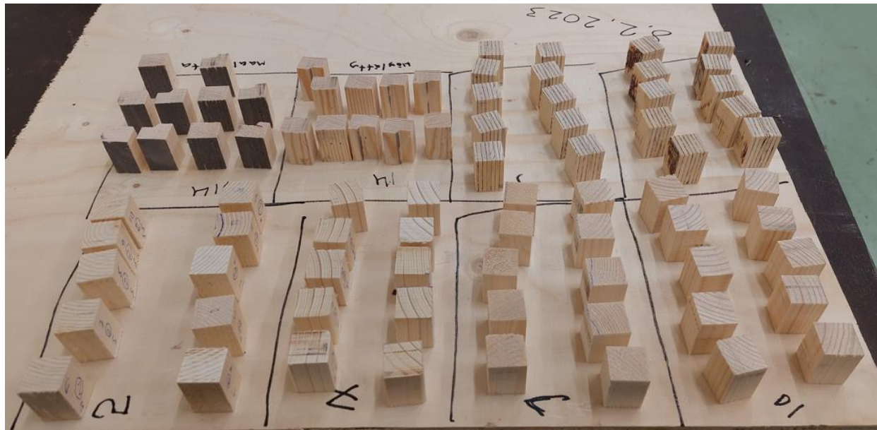
Figure 17 The 20 mm x 20 mm x 30 mm samples cut from the timber components for tests.
