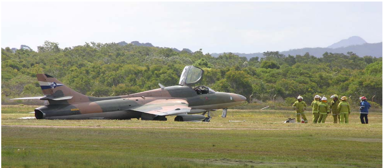
Hunter T75 accident (landing gear failure) in Australia in 2005. Source: Greg Weir. Copyright © 2006. www.airliners.net .
