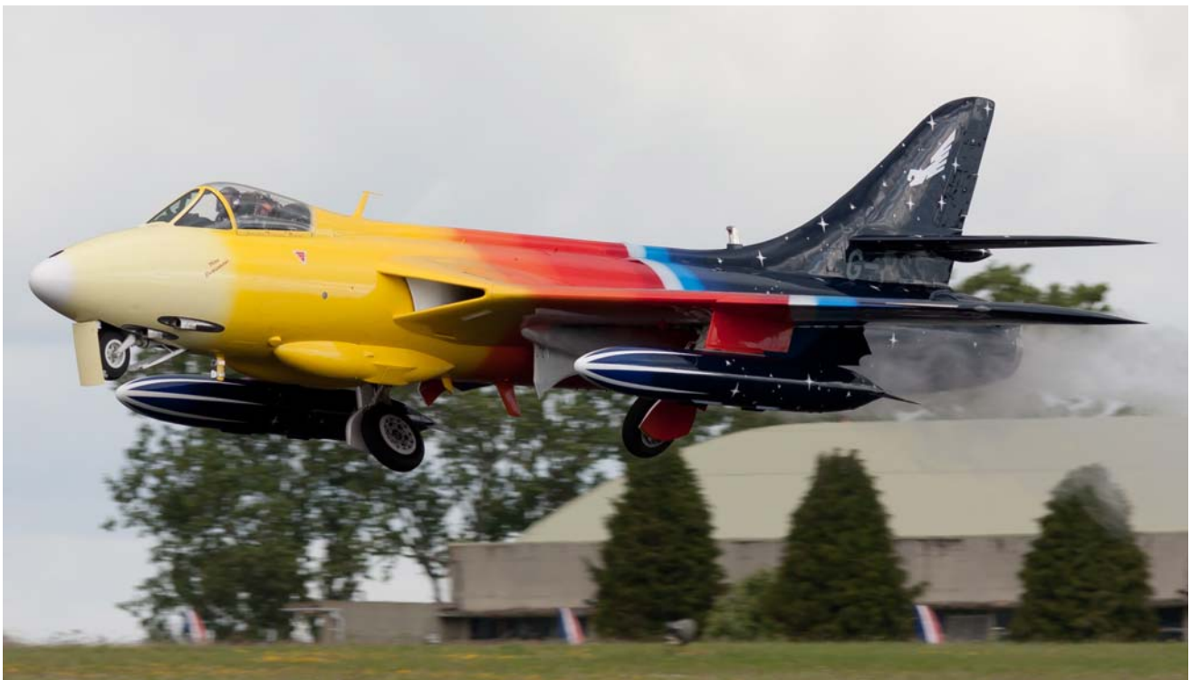
Hunter Mk.58 G-PSST accelerating during take-off at Kemble (UK) in June 2011. A rather significant amount of fuel is leaking and seen streaming. It was the result of a sticking refueling pressure relief valve. Source: Michael Brazier-Aviation-Images. Copyright © 2011. www.airliners.net . Below, another view of the incident a few instances later. Note the origin of the fuel leak forward of the white-painted fuselage gear door. Source: Max Hawkins. Copyright © 2011. www.airliners.net .
