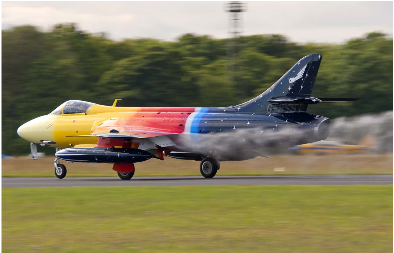
Hunter Mk.58 G-PSST accelerating during take-off at Kemble (UK) in June 2011. A rather significant amount of fuel is leaking and seen streaming. It was the result of a sticking refueling pressure relief valve. Source: Michael Brazier-Aviation-Images. Copyright © 2011. www.airliners.net . Below, another view of the incident a few instances later. Note the origin of the fuel leak forward of the white-painted fuselage gear door. Source: Max Hawkins. Copyright © 2011. www.airliners.net .
