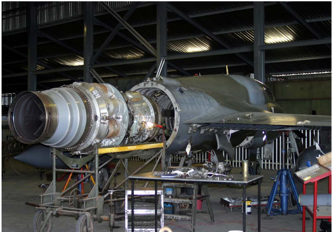
Rolls-Royce Avon 100 Series engine change on a Hunter T7 in South Africa. Source: Fanie Kleynhans. Copyright © 2003. www.airliners.net.
