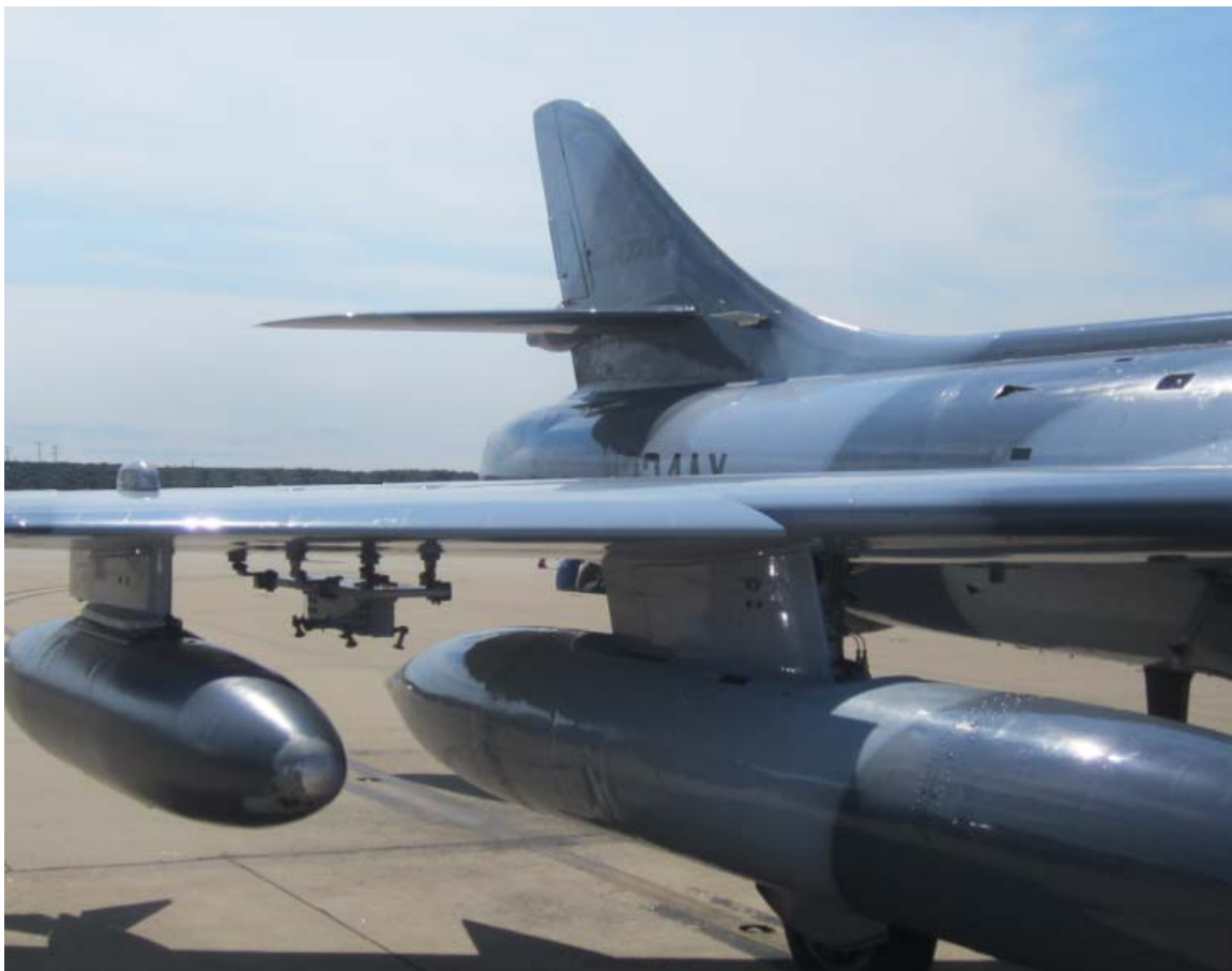
Hunter Mk. 58 close-ups - ACMI (Air Combat Maneuvering Instrumentation) pod and extra wing-mounted pylon. Source: FAA.
