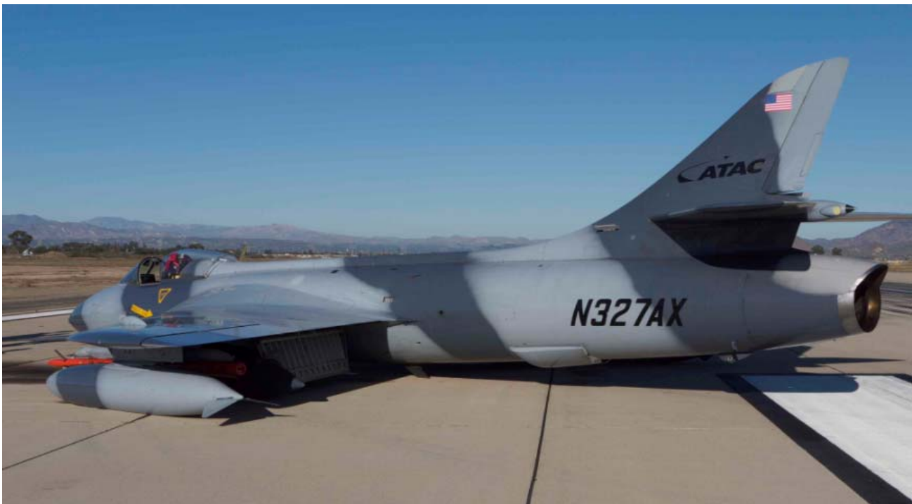
Hunter Mk. 58 gear-up landing, Pt. Mugu, California, 2012. Source: NTSB.
