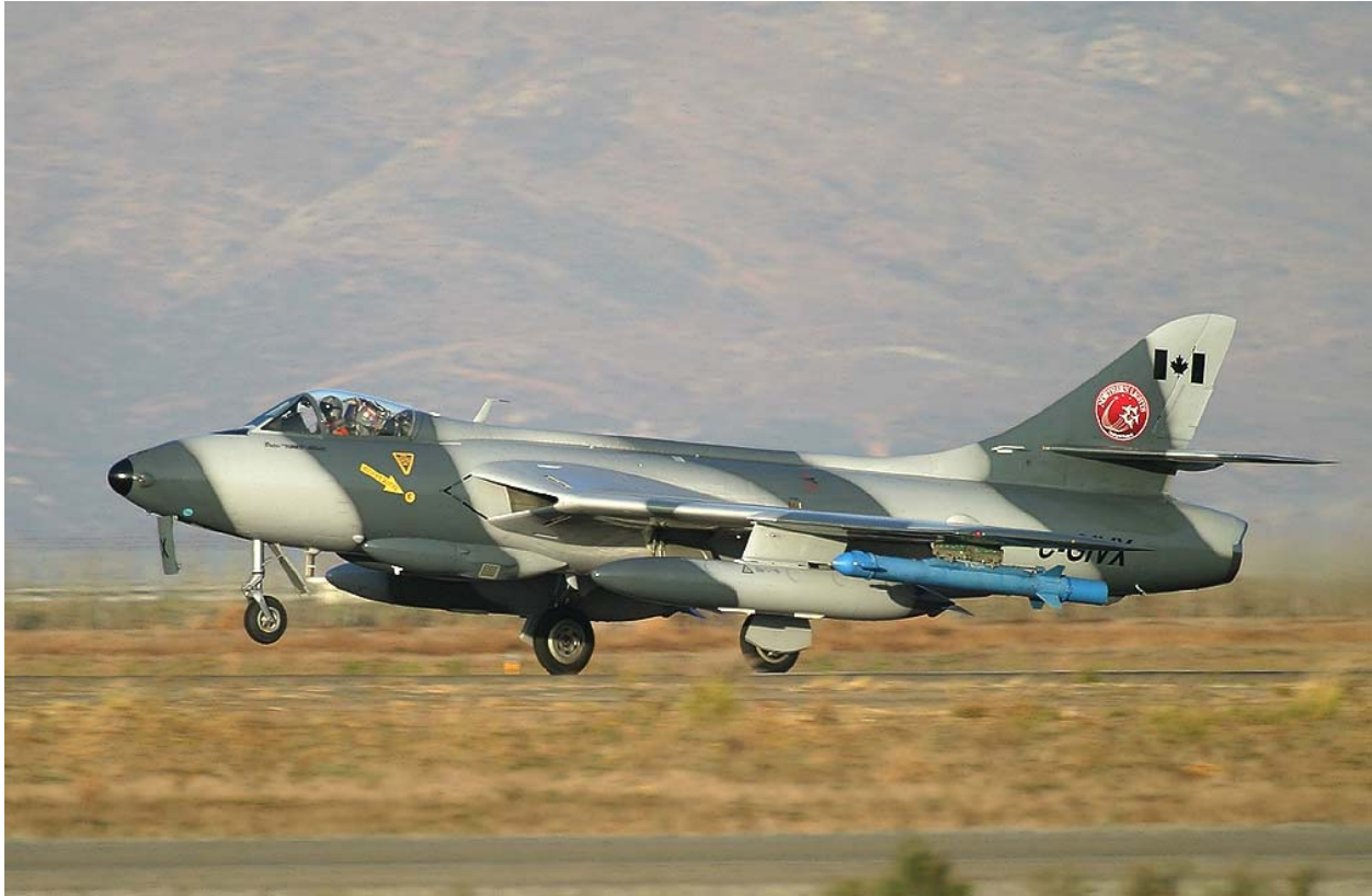
Canadian-registered Hunter Mk.58s belonging to Northern Lights Co. seen at Brown Municipal Airport (SDM), California, in December 2003. Above, one aircraft equipped with an ALQ-167 pod on the left outboard pylon. Below, two Hunters photographed during a formation take-off at Brown Municipal Airport. Source: Tony Zeljeznjak. Copyright © 2003. www.airliners.net .
