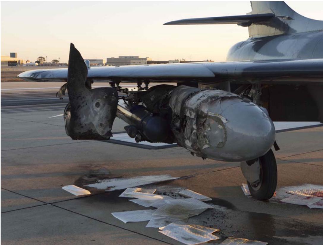
Hunter Mk. 58 gear-up landing, Pt. Mugu, California, 2012. Source: NTSB & FAA.
