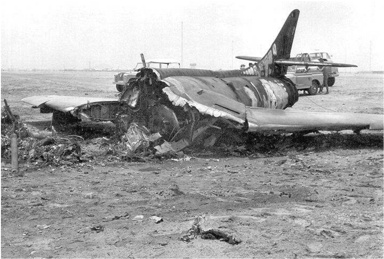
Aftermath of two RAF Hunter engine failure accidents in the 1960s. Source: Roger Wilkins via Ray Deacon. http://www.radfanhunters.co.uk
