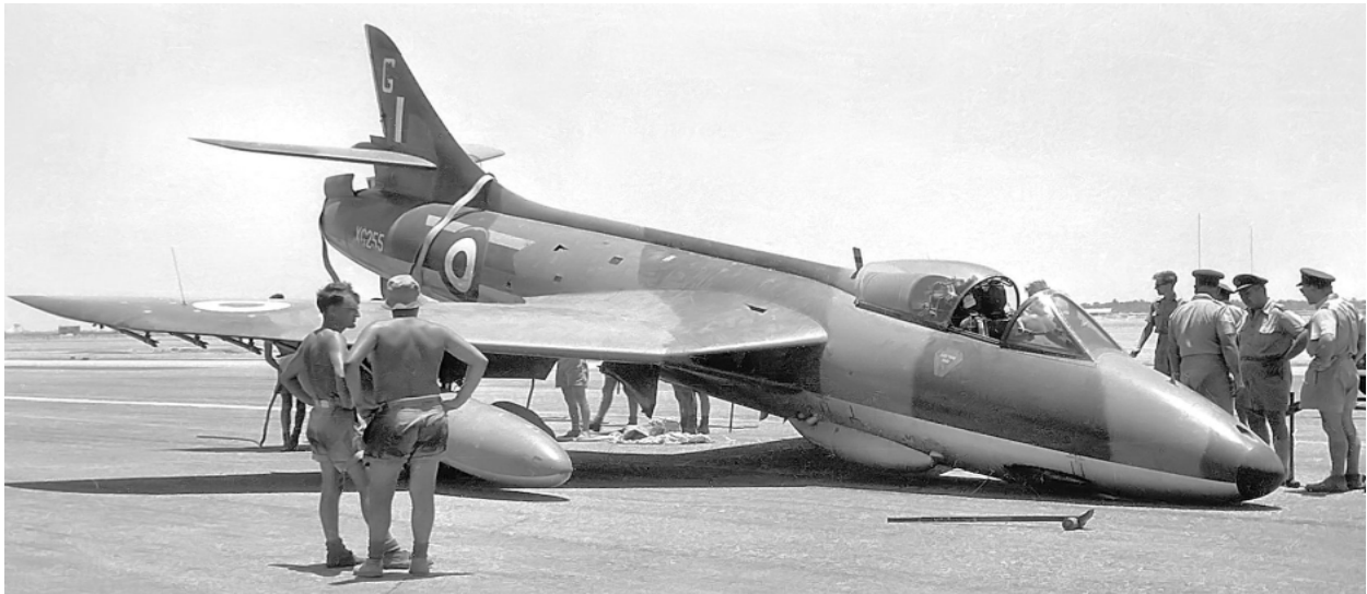
Typical Hunter accidents. Above, nose-gear failure. Below, external fuel tank separation. Source: Roger Wilkins via Ray Deacon. http://www.radfanhunters.co.uk .
