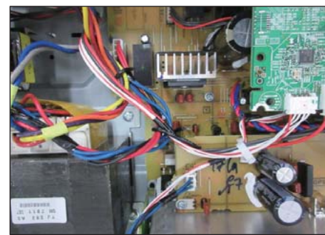
Fix with PN221 CB222-Power transformer CB581-Power transformer (V.P.S models) Fix with PN521 CB24-W2403 CB81-W5401 CB222-Power transformer
