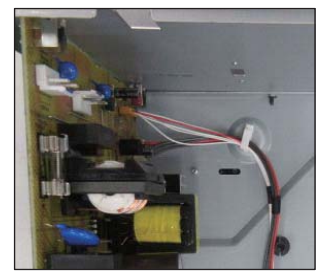
Fix with wire clam W5401 W5403
