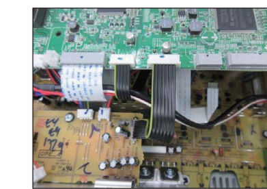
CB9540 must be inside the loop of CB22, CB27, CB25
