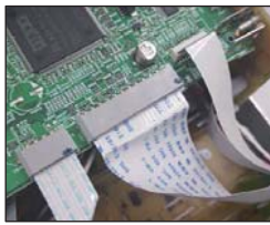
FFC 23p to OPERATION (1) (CB402)
