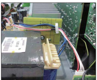
Fix with wire clamp Power transformer-CB524 CB477-W2111
