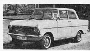
OPEL KADETT. A conventional car recently introduced by the German branch of General Motors, having a 993 c.c. engine developing 40 b.h.p. at 5,000 r.p.m. An all-synchromesh four-speed gearbox is used in this car which has been designed to compete against the Volkswagen 1200.
