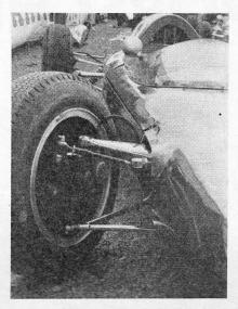
LOTUS front suspension. Springs and dampers have been taken inboard, though the gain in reducing drag must be trivial.
