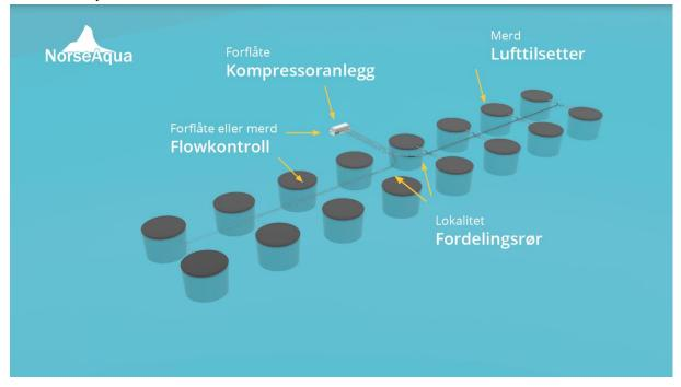
5.3.1 Aerator – Mid-Norwegian Ring The aerator distributes the compressed air in the water.
