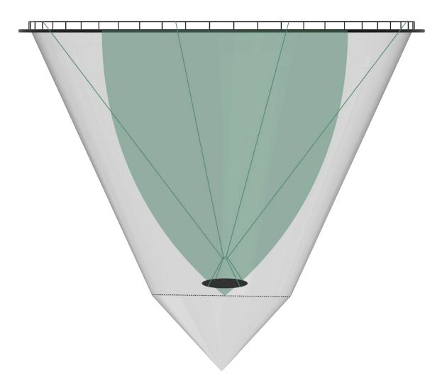
A coned net is the kind of net that is most likely to come into contact with the ring in strong currents. Therefore it is important that the following guidelines are followed:
