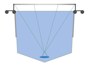
6.3.2 Fixing method 2 – Rope to a float
