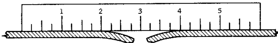
A. UNDER DIMPLED DIMPLE POORLY DEFINED
