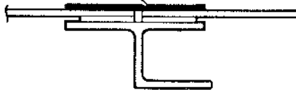
TYPICAL SEALING OVER FLOOR PANEL BUTT JOINTS
