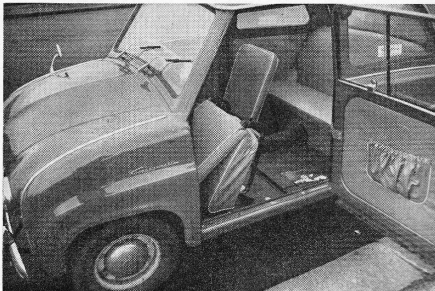
ACCOMMODATION is designed principally to provide a high degree of comfort for driver and front passenger. The rear seats are more suited for children, although four adults can be carried within the stressed skin body.
