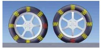
Also, checking the radial runout of the tire (when unloaded) does not give and indication of radial force fluctuations. The only method to accurately check for radial force variations is to use the GSP97BMW wheel balancer.
