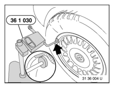
Excessive radial runout can caused conditions similar to a static imbalance. Radial force variations are also affected.
