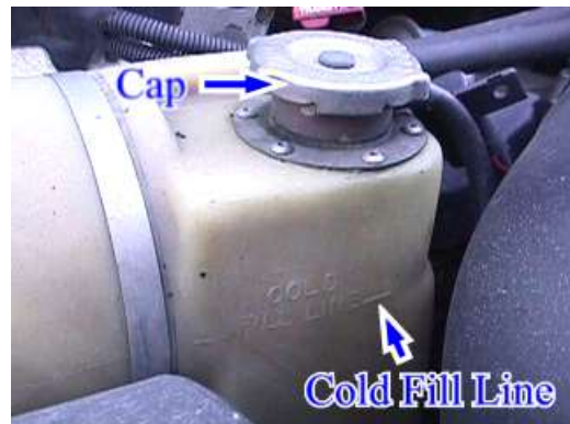
Illustration 2 – Surge Tank Cap and Fill Line
