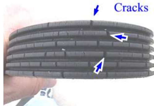
Illustration 1 – Minor Cracks in Serpentine Belt
