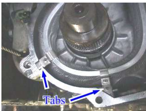
Illustration 5 – Updated Cooler Loop Installed
