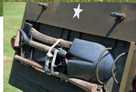
Standard army extras and cleverly designed stowage are a feature of this vehicle. Pioneer tools, two five-gallon liquid containers and a fire extinguisher were issued with each truck
