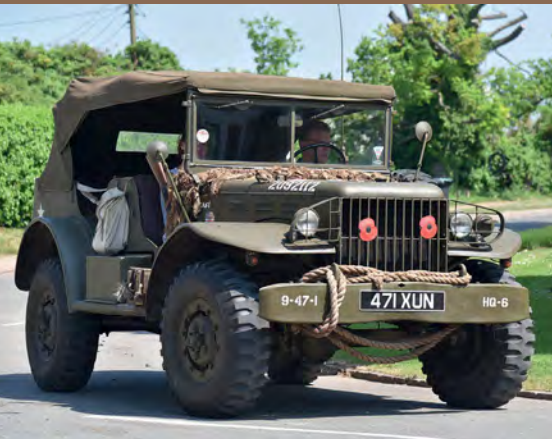
The three-quarter ton truck had a shorter cowl, a squared off and functional front end including the new design slatted but flat steel grilles
