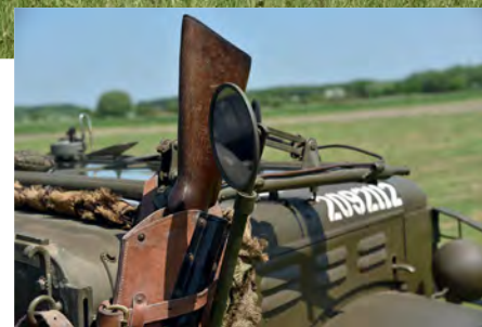
Many of the fixings and catches are often seen in polished brass but here they are correctly in Olive Drab - they were done this way so that they didn't catch the light
