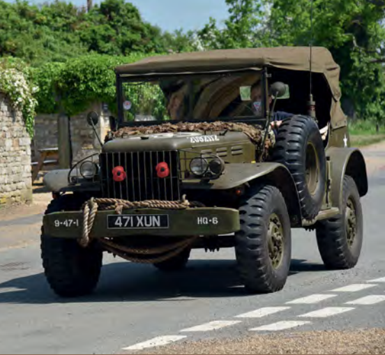
The Dodge WC series models had a side-mounted spare wheel, open sides and folding hood
