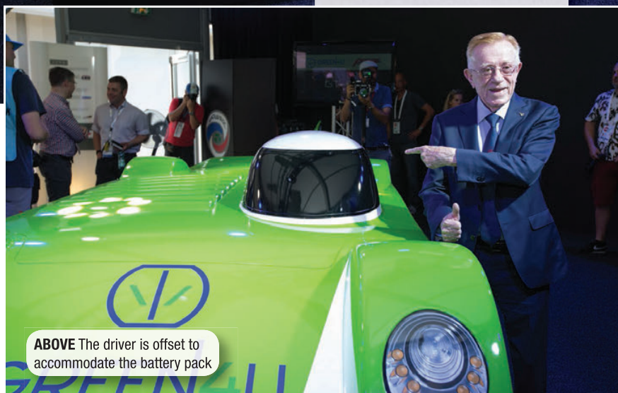
ABOVE Don Panoz considers the Green4U Panoz Racing GT-EV, an all-electric racecar designed to compete with ICE rivals, to be the 'Holy Grail' of racing
