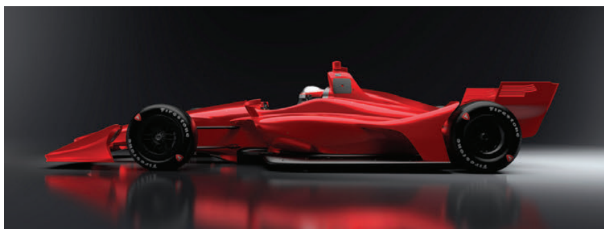
ABOVE & BELOW IndyCar based its new car on a form of reverse-engineering: it worked on aesthetics first, then created a performance package around it. This is the Road/Street and Short Oval kit seen in CAD (above) and the Superspeedway trim (below)
