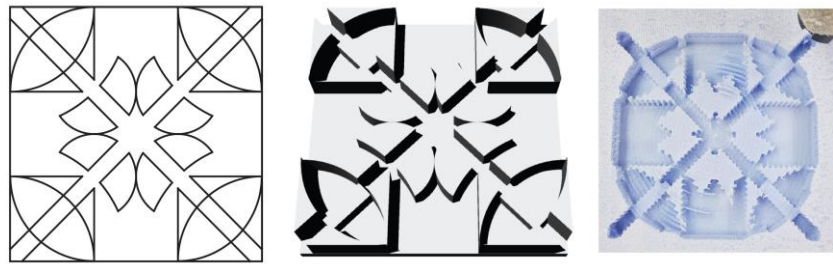
Figure 4: Three stages of the model generation (from left): Generating a 2d pattern, 3d modeling of a surface based on the pattern, CNC-milled material outcome (Image courtesy: Nazlı Bahar Ursavaş)
