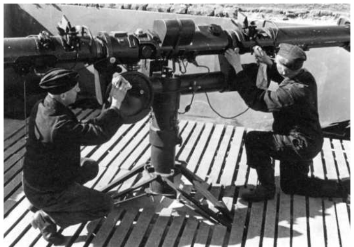
■ The 4-metre rangefinder used by heavy flak units combined with a fire control computer made the 88mm flak gun accurate and deadly. One of the units is seen here on a Siebel Ferry.
