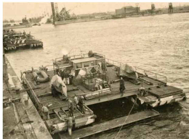
■ A Siebel Ferry fitted-out with two 88mm anti-aircraft guns. Moored behind are Siebel Ferries equipped with aircraft engine propulsion units.
