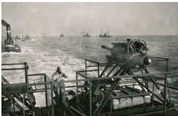
■ A clear view of the BMW VI aircraft engine used on a transport Siebel ferry. These were so loud they were eventually removed because it was impossible to hear orders. Noteworthy in this image is the crew member holding his fingers in his ears! In the background are the tugs that would have been used to tow these ferries to the English coast.
