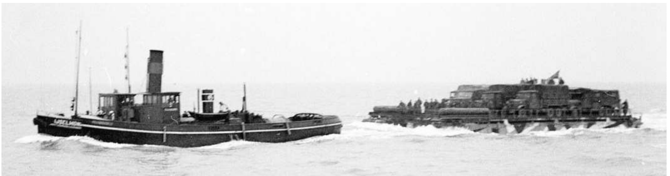
■ A fully loaded Siebel Ferry pulled by a tug which was to bring the ferries across the English Channel where the craft's own engines would then bring them to the beaches to unload. This ferry is loaded with trucks and men.
