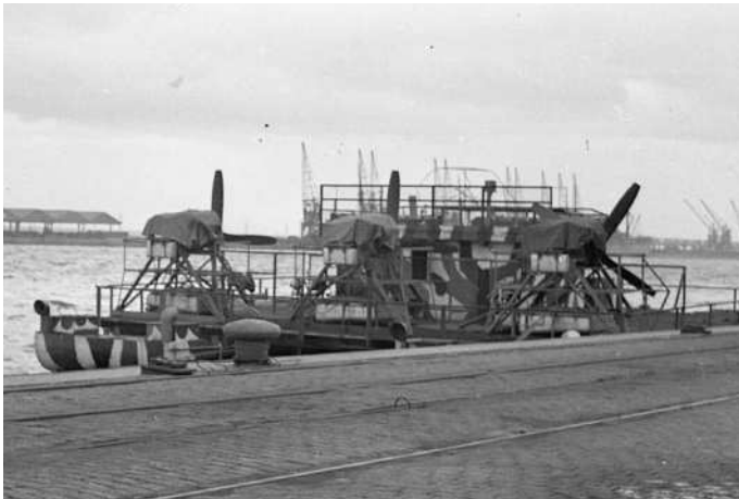
■ This Siebel Ferry has three BMW VI aircraft engines with propellers mounted above the ferry for additional power and directional control. These engines were so loud that no voice commands were possible. They were eventually phased out.
