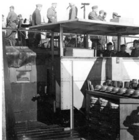
■ Left: The wheelhouse on a heavy flak Siebel ferry. Note the storage for the 88mm anti-aircraft shells in their wickerwork baskets forward of the pilot house, stowed below the steel helmets and gasmask cases.
